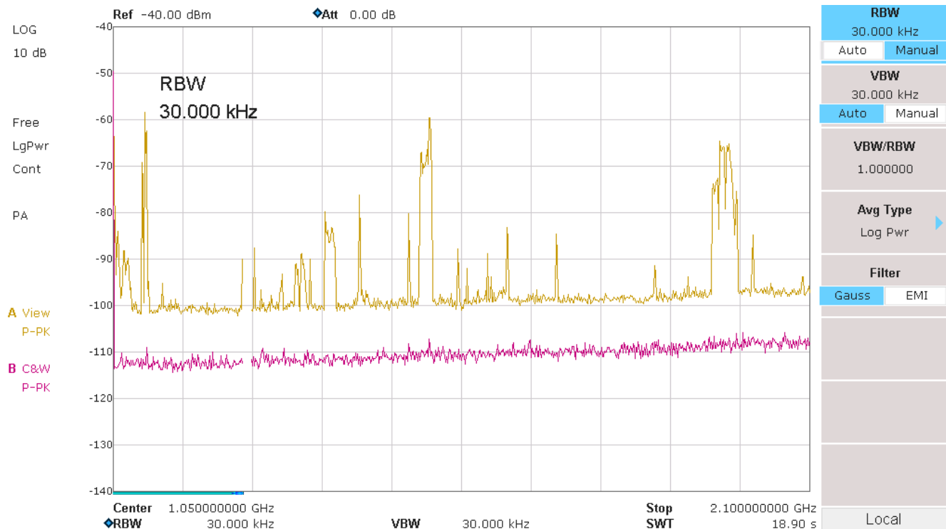
Picture 19: ambient noise picked up by the TBTC1 TEM-cell (set up according to picture 2)
