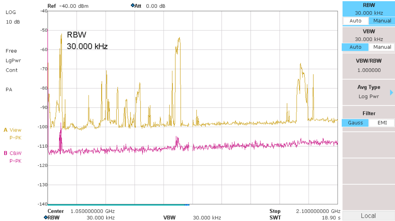
Picture 20: ambient noise picked up by the conducted noise test set up (set up according to picture 5)
