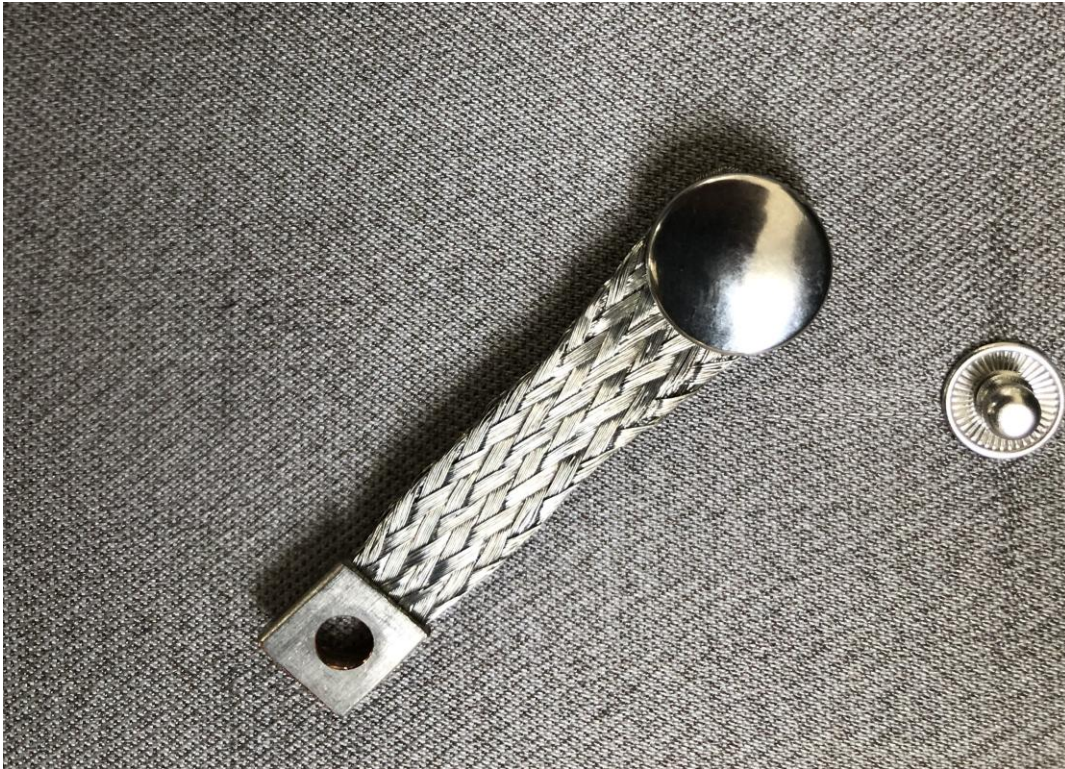
Picture 4: using textile rivets to establish electrical contact to the ground plane
