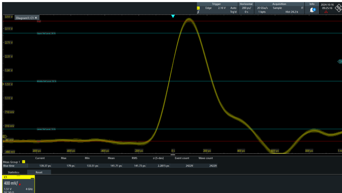
Picture 7: output pulse, 20 MHz base frequency, 50 \Omega termination
