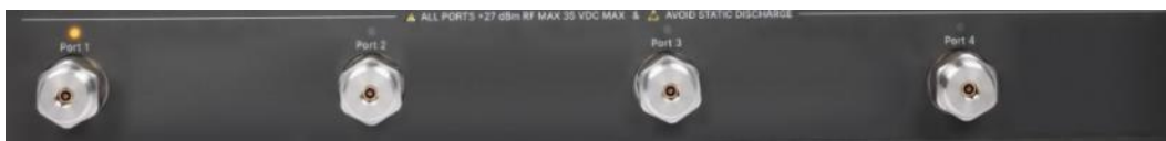
Figure 5-7 Front panel RF connectors (4-port VNA)
