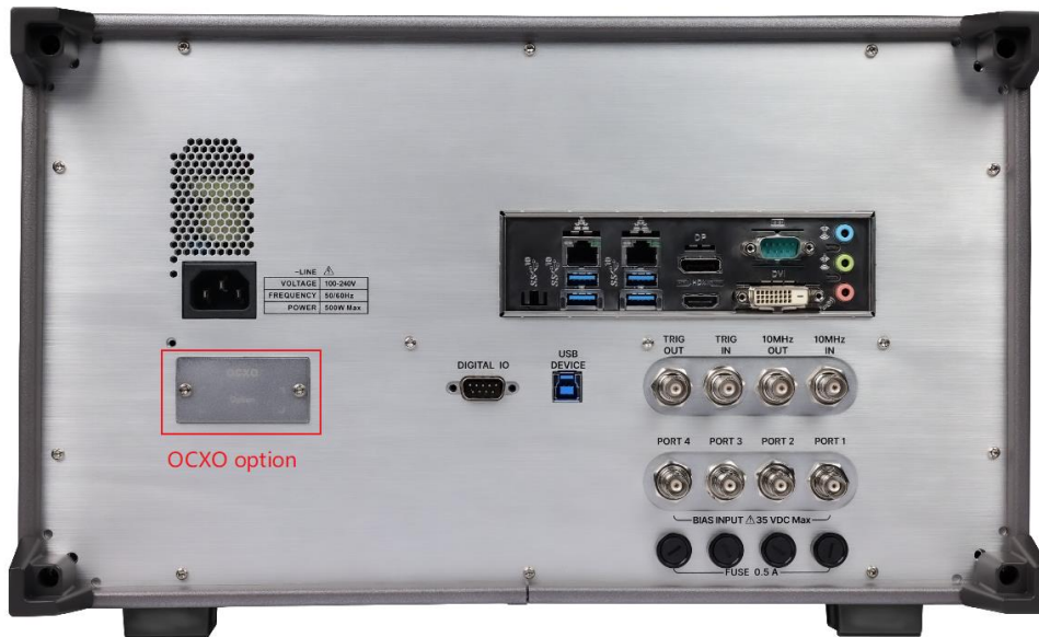
Figure 5-11 OCXO option installation guide
