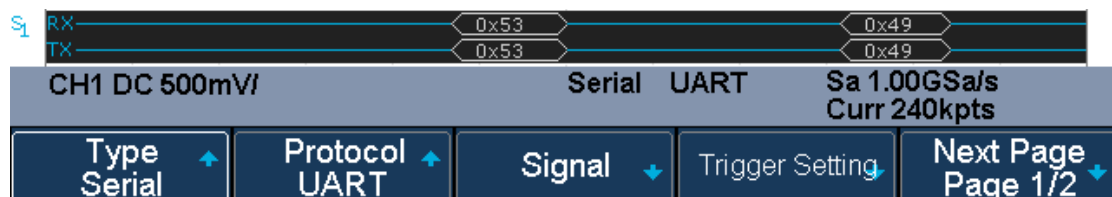
Figure 53 UART Decode Bus Display
