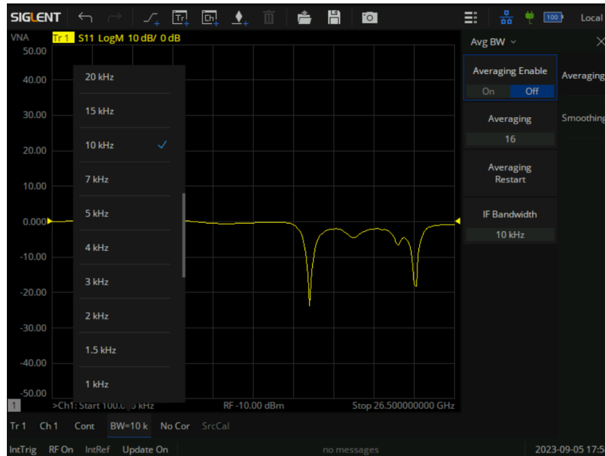
Figure 5-8 Set the IF from the status bar
