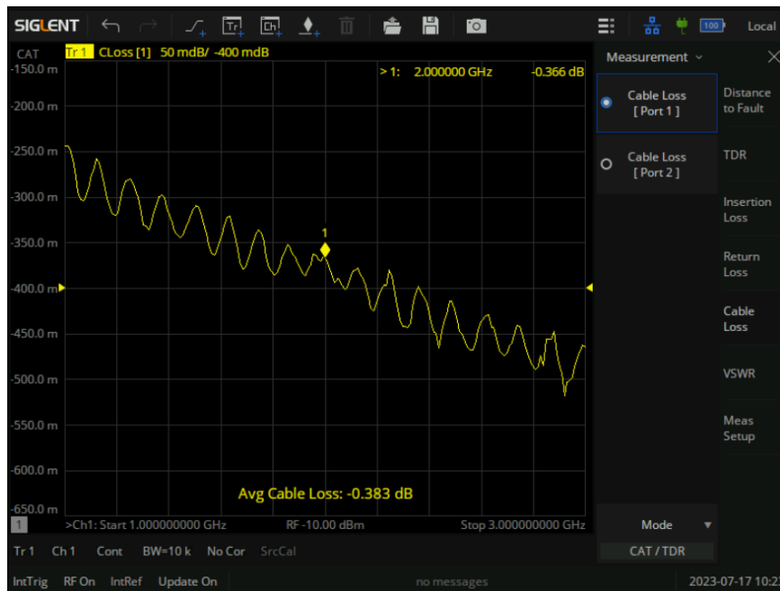
Figure 11-8 Cable loss measurement interface
