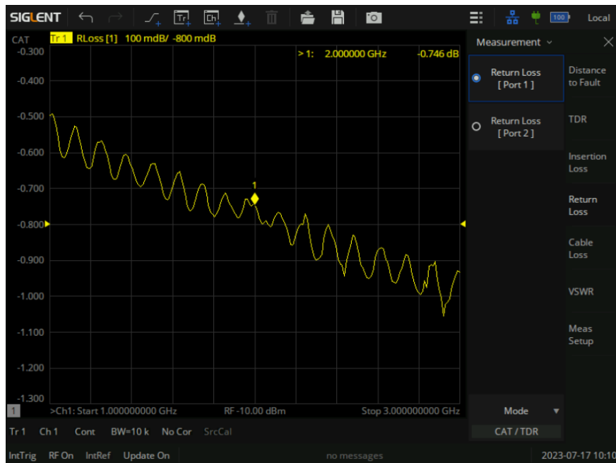
Figure 11-7 Return loss measurement interface
