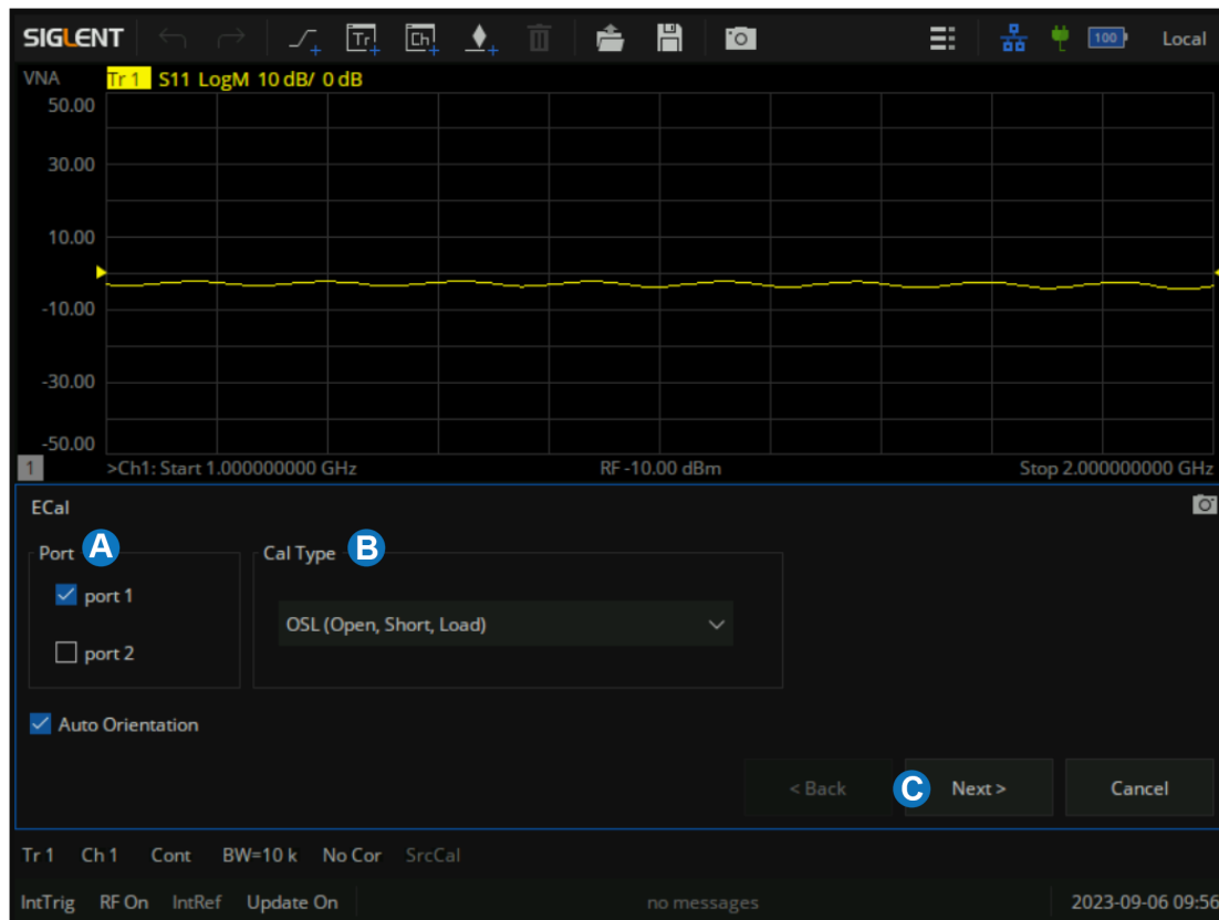
Figure 6-40 ECal config menu
