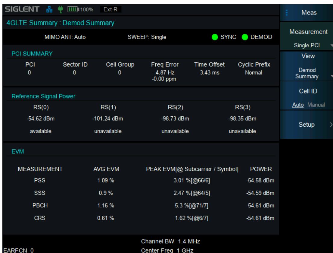
Figure 9–1 Single PCI Demodulation View
