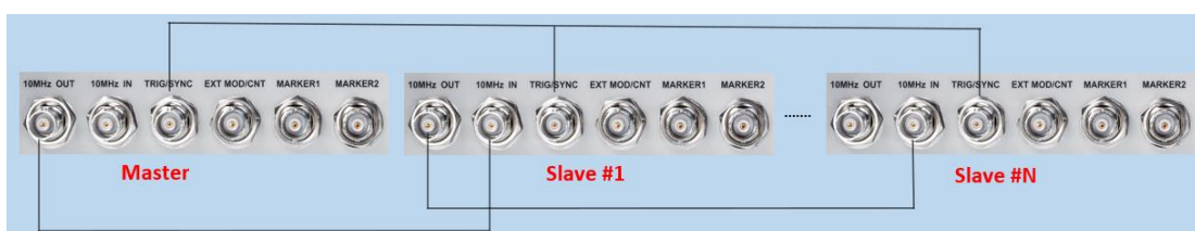
Figure 17-1 wiring diagram of multi-device synchronization
