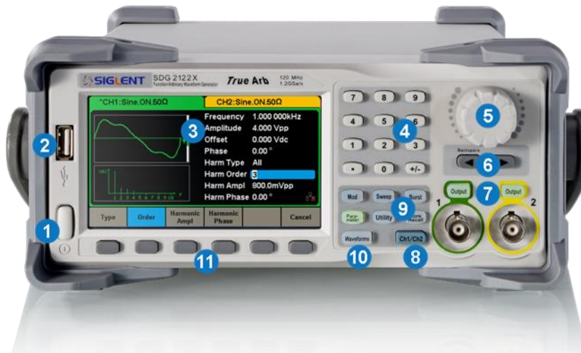
Figure 2 SDG2000X Front Panel
