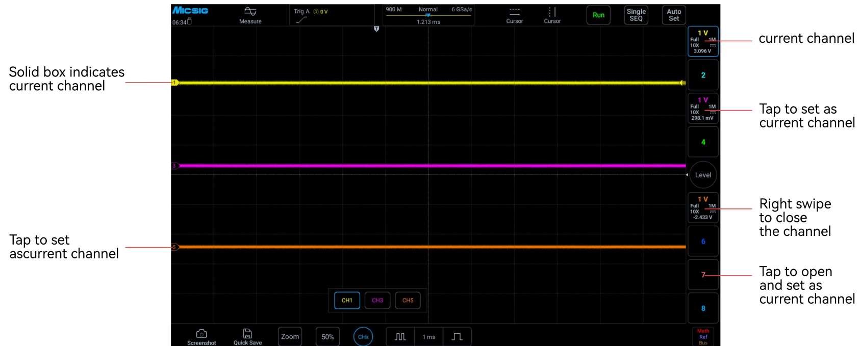
Figure 5-4 Channel Open, Close and Switching
