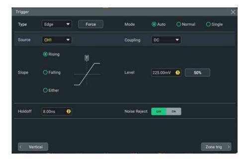
Figure 8.1 Trigger System Menu
