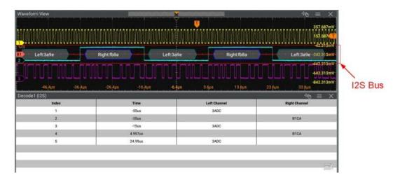
Figure 19.19 I2S Decoding Event Table
