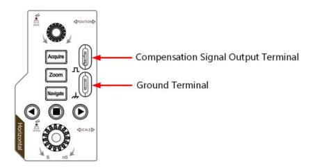
Figure 4.13 Use the Compensation Signal
