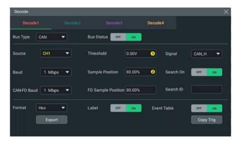
Figure 19.13 CAN Decoding Menu
