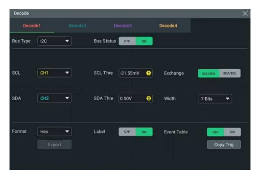
Figure 19.8 I2C Decoding Menu
