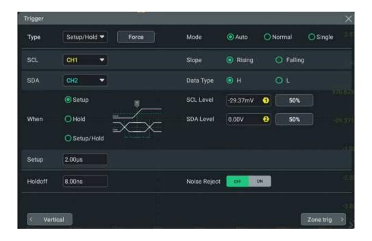
Figure 8.23 Setup/Hold Trigger Setting Menu
