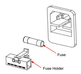
Figure 4.8 Replace the Fuse
