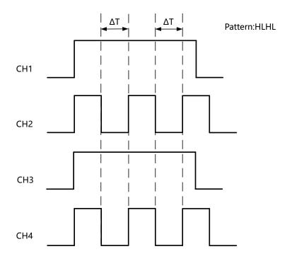
**Figure 8.12 Duration Trigger**
