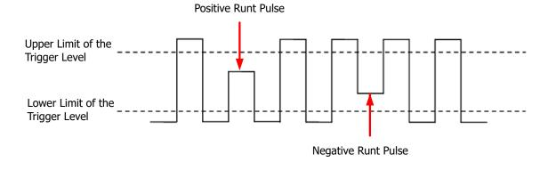
Figure 8.17 Runt Trigger
