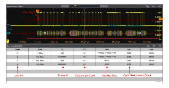
Figure 19.15 CAN Decoding Event Table
