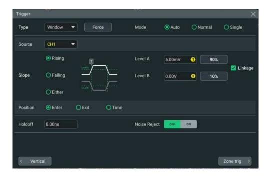
Figure 8.19 Window Trigger Setting Menu
