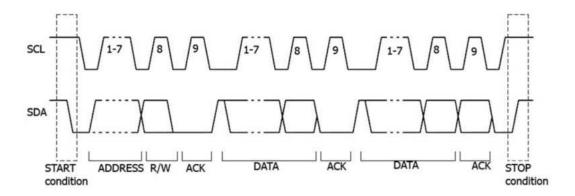
Figure 8.28 Sequential Chart of I2C Bus
