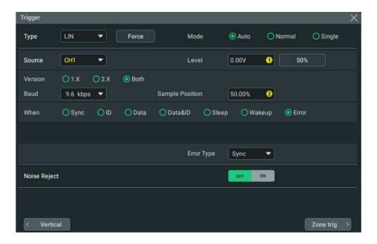
Figure 8.40 LIN Trigger Setting Menu
