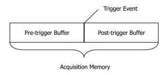
Figure 8.2 Schematic Diagram of the Acquisition Memory
