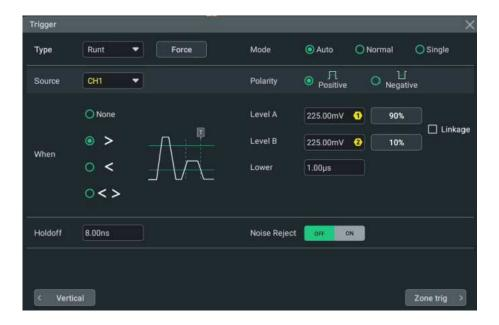
Figure 8.18 Runt Trigger Setting Menu
