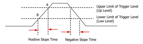
Figure 8.6 Positive Slope Time/Negative Slope Time
