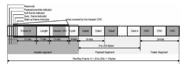
Figure 8.37 Frame Format of FlexRay Bus
