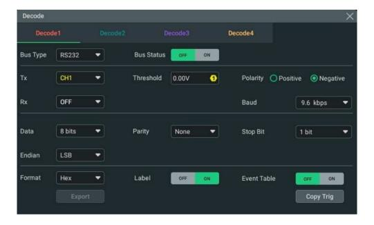
Figure 19.5 RS232 Decoding Menu
