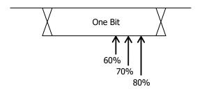
Figure 8.36 Sample Position (CAN Trigger)
