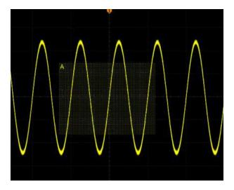
If you enable Zone A, select CH1 as the source for Zone A, select "Not intersect" as the condition, the following figure is displayed.
