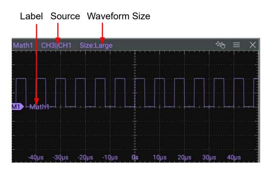
Figure 9.10 Logic Operation Result Display Window
