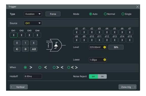
Figure 8.13 Duration Trigger Setting Menu of MHO Series 4-CH Model
