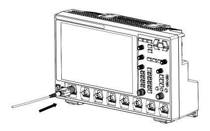
**Figure 4.9 Connect the Passive Probe**
