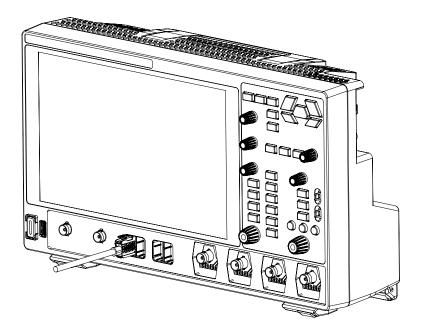
**Figure 4.12 Connect the Logic Probe**
