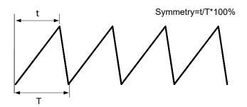
Click or tap the of input field of **Symm** to set the symmetry with the pop-up numeric keypad. You can also use the specified knob indicated in the input field to set it. The available range of symmetry is from 0.1% to 99.9%. By default, it is is 50%.
