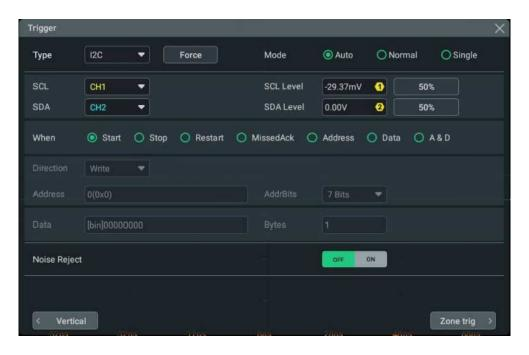
Figure 8.29 I2C Trigger Setting Menu
