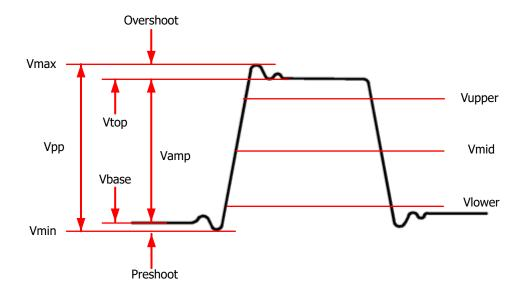
Figure 10.3 Voltage Parameters
