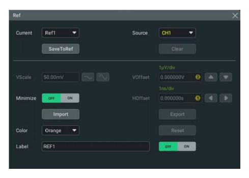
Figure 17.1 Reference Waveform Menu
