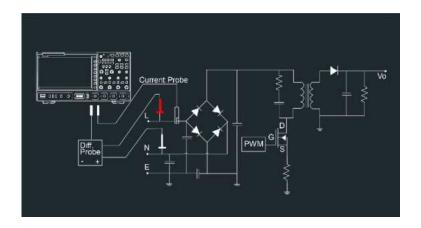
**Figure 16.3 Connection Diagram of Power Quality Analysis**
