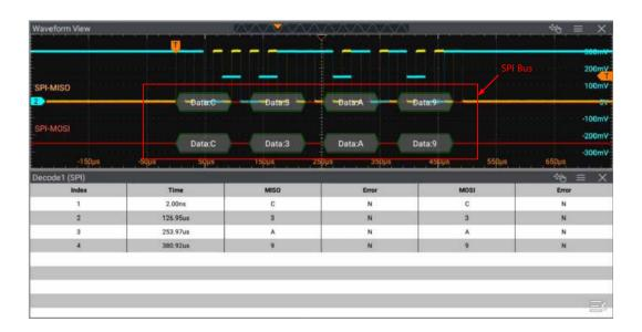
Figure 19.12 SPI Decoding Event Table
