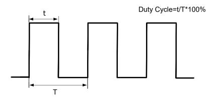
Click or tap the of input field of **Duty** to set the duty cycle with the pop-up numeric keypad. You can also use the specified knob indicated in the input field to set it. The available range of duty cycle is from 1% to 99%. By default, it is 50%.
