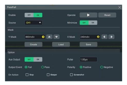
Figure 18.1 Pass/Fail Test Menu
