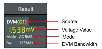
The voltage value above shows the measurement extrema over the last 3 seconds.
