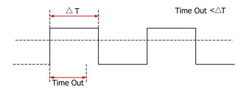
**Figure 8.15 Timeout Trigger**
