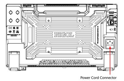
Figure 4.7 Connect to AC Power
