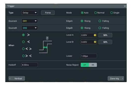
Figure 8.21 Delay Trigger Setting Menu
