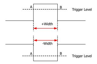
Figure 8.4 Positive/Negative Pulse Width
