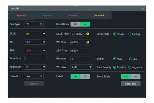
Figure 19.18 I2S Decoding Menu
