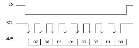
Figure 8.32 Sequential Chart of SPI Bus
