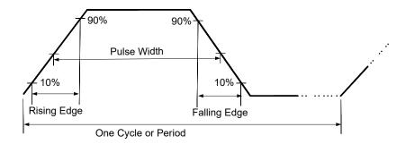
Click or tap the input field of **Rise Edge** to set the pulse rising edge time. Click or tap the input field of **Fall Edge** to set the pulse falling edge time with the pop-up numeric keypad. You also use the specified knob indicated in the input field to set the rising and falling edge time. The rising/falling edge time ranges from 1 ps to 1 s. By default, it is 300 ps.
