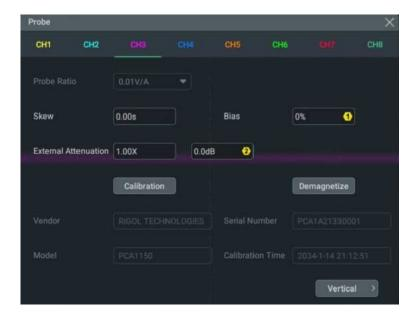
**Figure 5.5 Active Probe Setting Menu**
