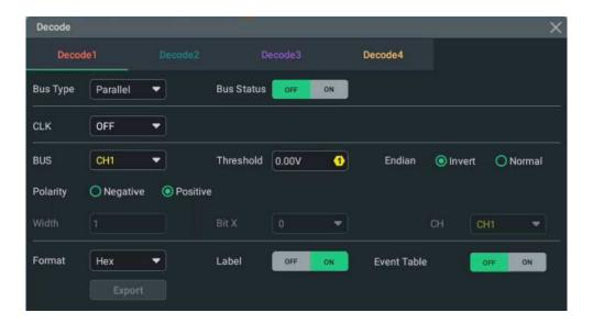
Figure 19.2 Parallel Decoding Menu
