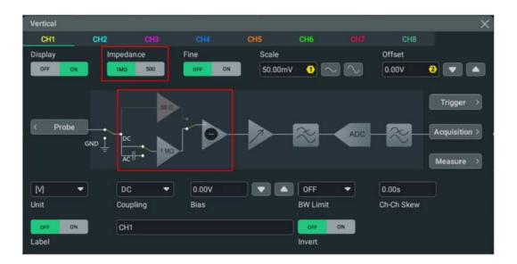
Figure 5.2 Input Impedance Switchover
