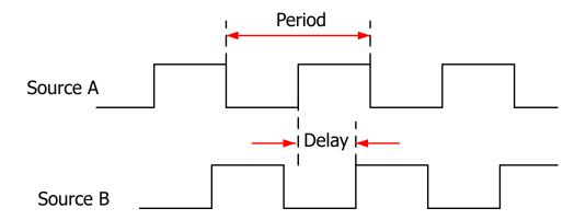
**Figure 10.2 Delay and Phase Parameters**
