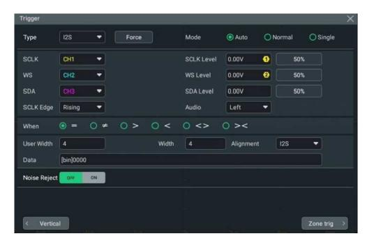
Figure 8.43 I2S Trigger Setting Menu
