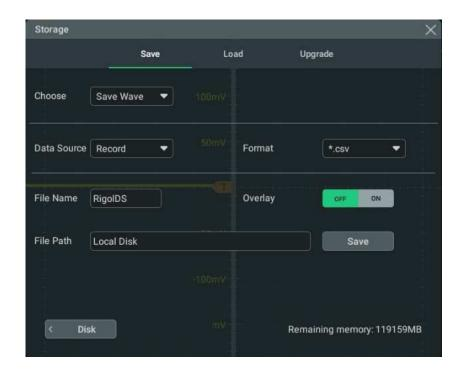
**Figure 24.2 Waveform Saving Setting Menu**
