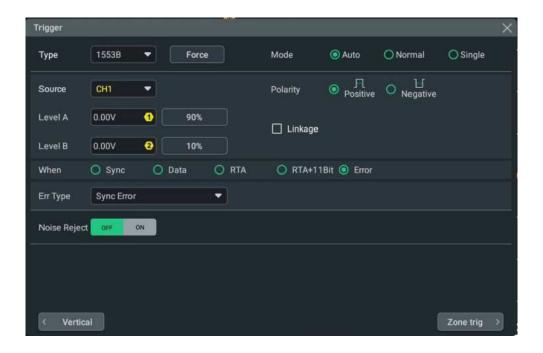
Figure 8.45 MIL-STD-1553 Trigger Setting Menu
