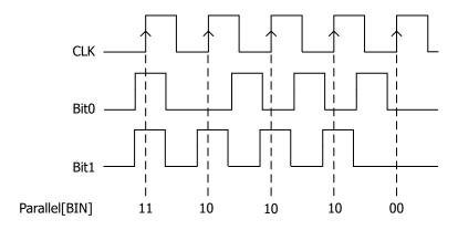
Figure 19.1 Schematic Diagram of Parallel Decoding
