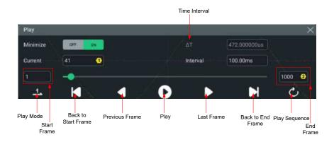
Figure 21.2 Minimized Window of Play Operation Interface
