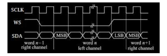
Figure 8.42 Sequential Chart of I2S Bus
