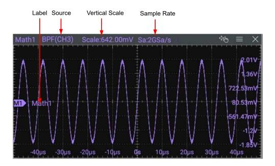
Figure 9.5 Function Operation Result Display Window
