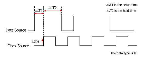
Figure 8.22 Setup/Hold Trigger
