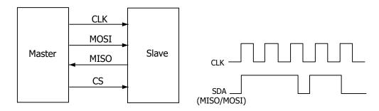
Figure 19.10 SPI Serial Bus
