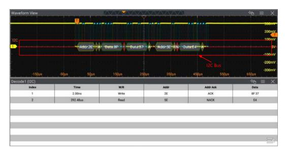
**Figure 19.9 I2C Decoding Event Table**
