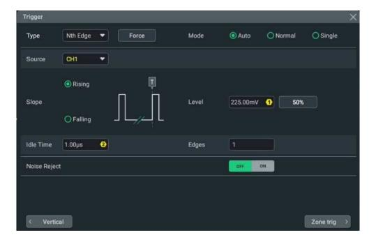
Figure 8.25 Nth Edge Trigger Setting Menu
