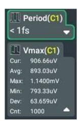
Figure 10.5 Display Statistics at the Right Section of the Screen
