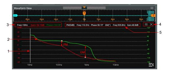
Figure 15.3 Bode Plot Displayed in Waveform Display Form
