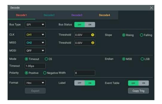
Figure 19.11 SPI Decoding Menu
