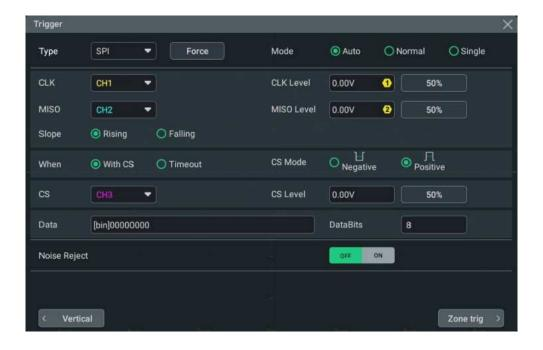
Figure 8.33 SPI Trigger Setting Menu
