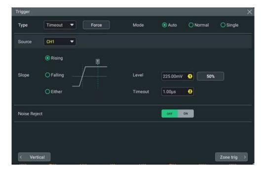
Figure 8.16 Timeout Trigger Menu
