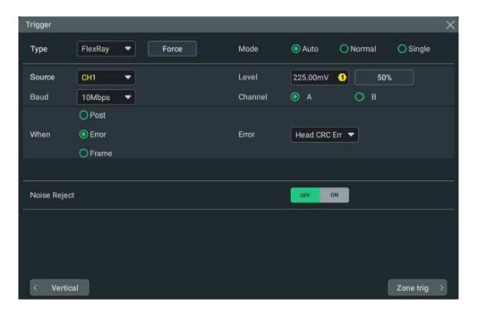
Figure 8.38 FlexRay Trigger Setting Menu
