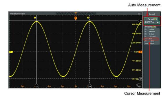
**Figure 10.8 Manual Cursor Measurement Example**
