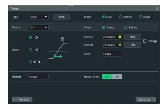
**Figure 8.7 Slope Trigger Setting Menu**
