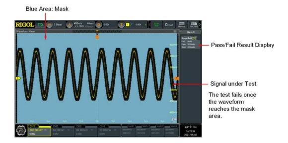
Figure 18.2 Pass/Fail Test Interface
