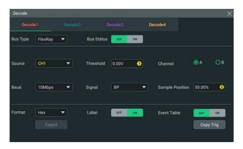
Figure 19.20 FlexRay Decoding Menu
