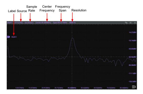
Figure 9.7 FFT Operation Result Display Window
