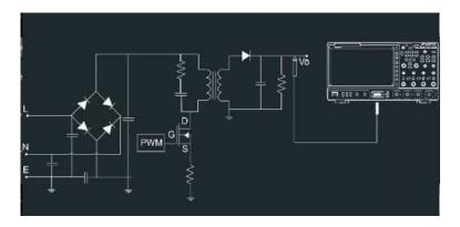
**Figure 16.5 Connection Diagram of Ripple Analysis**
