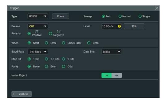
Figure 8.27 RS232 Trigger Setting Menu
