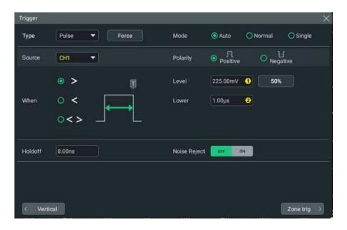
Figure 8.5 Pulse Trigger Setting Menu
