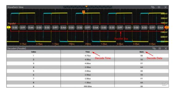
**Figure 19.3 Parallel Decoding Event Table**
