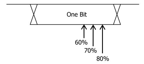
Figure 8.41 Sample Position (LIN Trigger)
