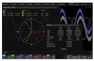
The Power Analysis and TPPA (3-phase Power Analysis) options provides a full suite of power measurements and analysis, which greatly improve the measurement efficiency in switching power supplies and power devices design. Combining the TPPA option with the 6/8 channels oscilloscope, high-voltage differential probes and current probes, we provide a complete solution of 3-phase power analysis
