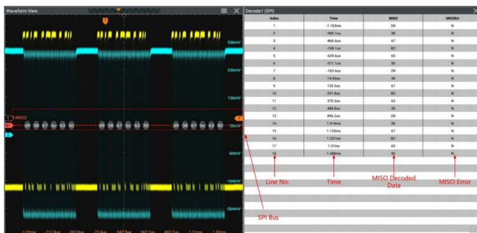
Figure 18.13 SPI Decoding Event Table
