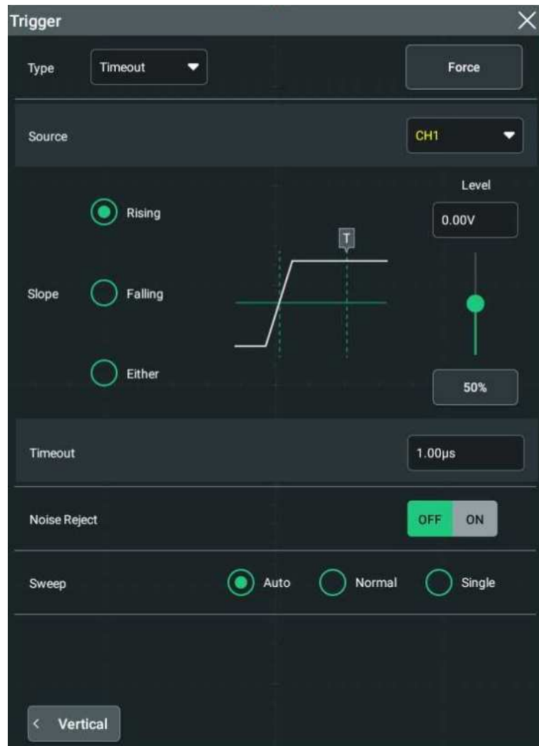
Figure 8.14 Timeout Trigger Menu
