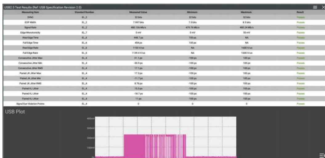
Figure 19.2 USB2.0 Signal Quality Compliance Analysis Test Result
