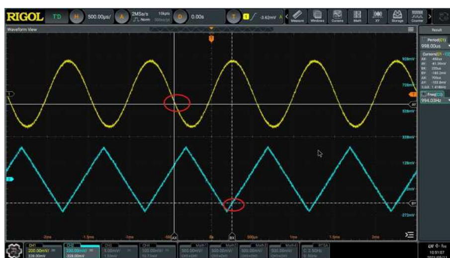
Figure 10.13 Track Measurement (before Horizontal Expansion)
