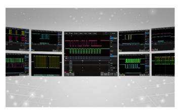
Display the decoded characters through the events list. Bus protocol information can be quickly and intuitively displayed in tabular form. I2C, SPI, UART, CAN, LIN, CAN FD, FlexRay, I2S, MIL-STD-1553B, SENT, Manchester, ARINC429 and USB 2.0 are supported
