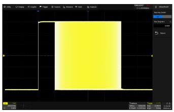
Segmented memory collection will store the waveform into multiple memory segments (up to 80,000) and each segment will store a triggered waveform as well the dead time information. The interval between segments can be as small as 1.3 µs. All of the segments can be played back using the History function
