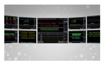
Display the decoded characters through the events list. Bus protocol information can be quickly and intuitively displayed in tabular form. I2C, SPI, UART, CAN, LIN, CAN FD, FlexRay, I2S, MIL-STD-1553B, SENT, Manchester and ARINC429 are supported
