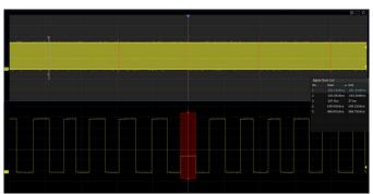
SignalScan automatically searches events by software according to the search conditions set by users, and marks them. Different from hardware search, in SignalScan the supported search conditions are richer, while the scan speed is relatively slower
