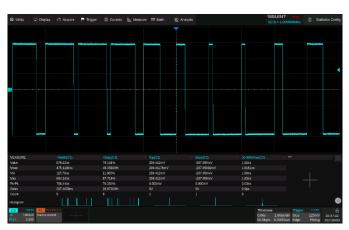
Statistics show the current value, maximum value, minimum value, standard deviation, and mean value of up to 12 parameters simultaneously. A histogram is available to show the probability distribution of a parameter. Trend and Track are available to show the parameter value vs. time.
