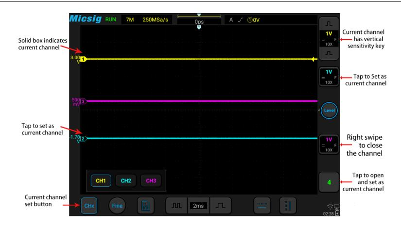
Figure 5-4 Channel Open, Close and Switching
