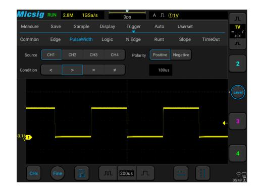
Figure 6-14 Pulse Width Trigger Setting Menu
