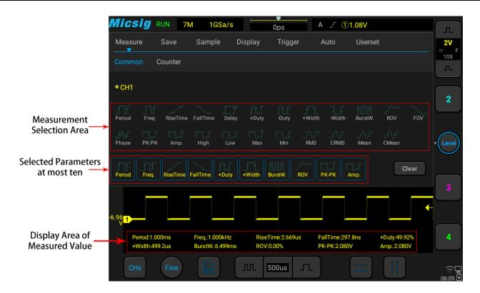
Figure 7-1 Automatic Measurement Menu
