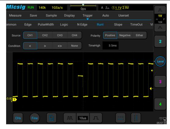
Figure 6-25 Runt Trigger Setting Menu
