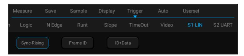
Figure 12-11 LIN Trigger Mode Configuration Menu
