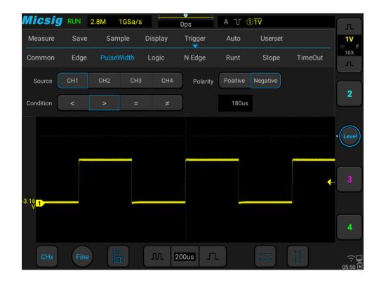
Figure 6-15 Negative Polarity Pulse Level Flip
