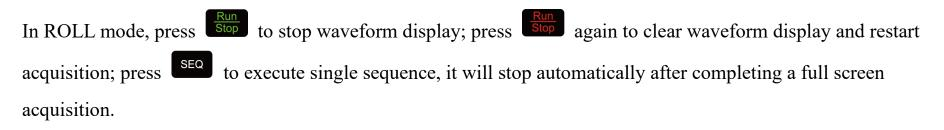
ROLL mode is generally used to observe waveforms with frequencies below 5 Hz.
