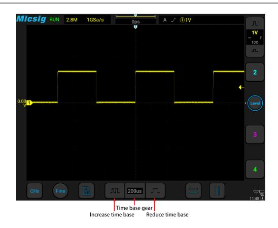
Figure 4-3 Adjust the Horizontal Time Base
