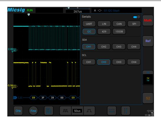
Figure 12-22 I2C Bus Configuration Menu
