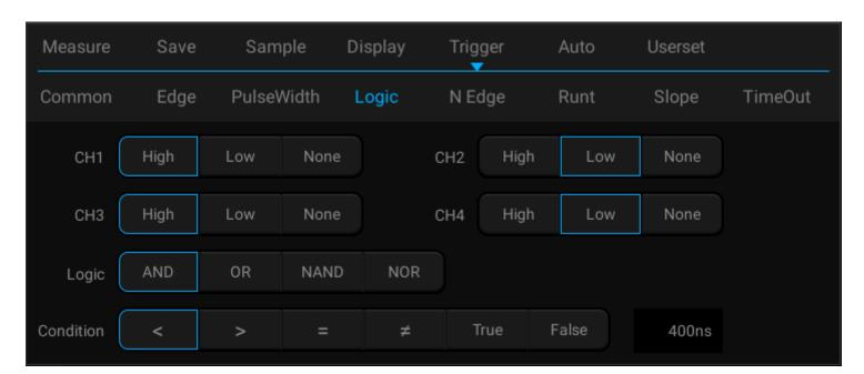
Figure 6-21 Logic Trigger Setting Menu
