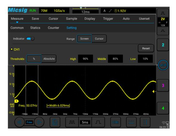
Figure 7-13 Set Middle Thresholds as 80%
