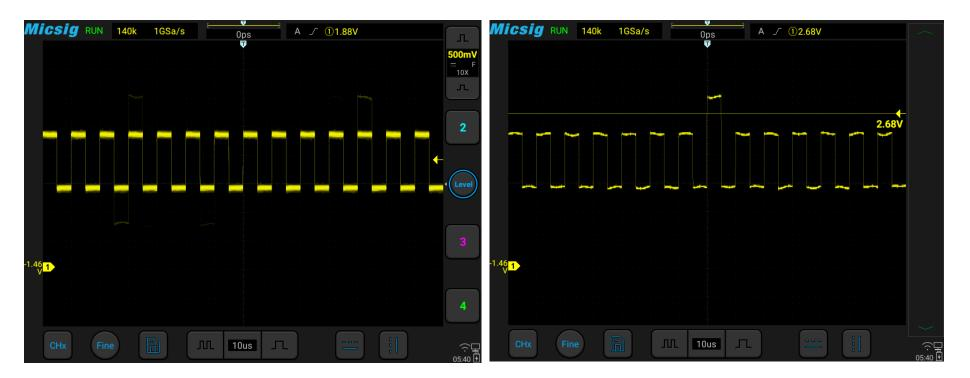
Figure 6-3 Abnormal Signal in Periodic Signals
