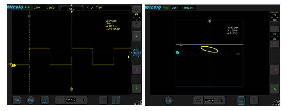
Figure 7-18 Cursor Measurement Pulse Width
