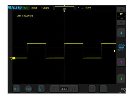
Figure 7-15 Frequency Meter Measurement
