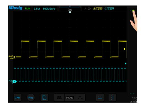
Figure 6-22 Trigger Level Adjustment
