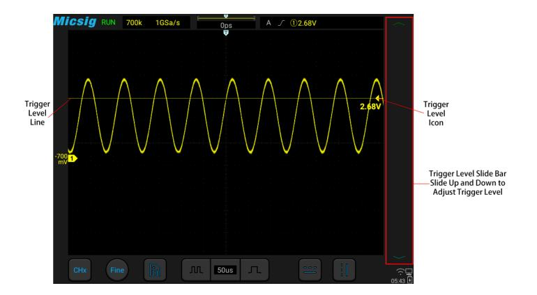
Figure 6-8 Trigger Level
