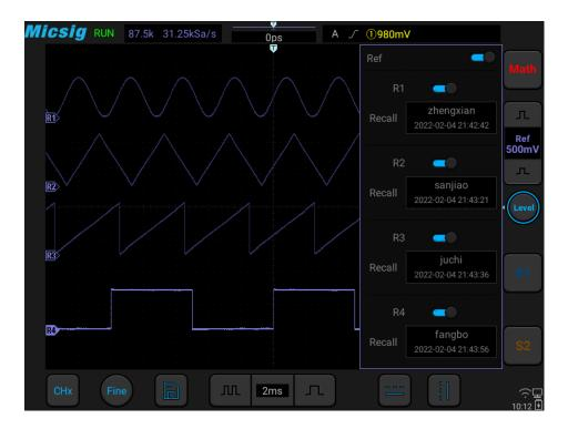
Figure 9-7 Restore Reference Waveform
