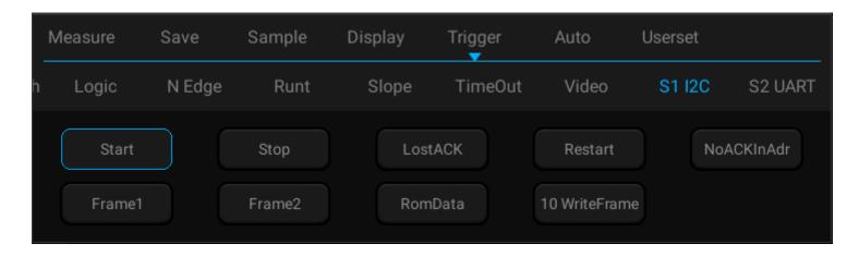
Figure 12-23 I2C Trigger Mode Configuration Menu
