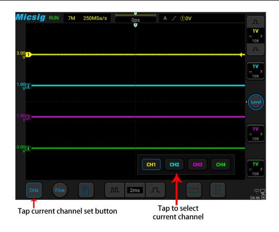
Figure 5-5 Using the Current Channel Selection Button
