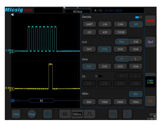
Figure 12-18 SPI Bus Configuration Menu
