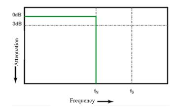
Figure 11-2 Theoretical Brick-Wall Frequency Response
