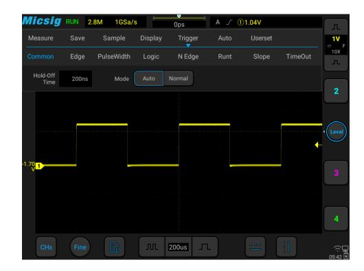
Figure 6-5 Oscilloscope Trigger Mode Setting
