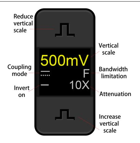
Figure 5-3 Channel Display Interface
