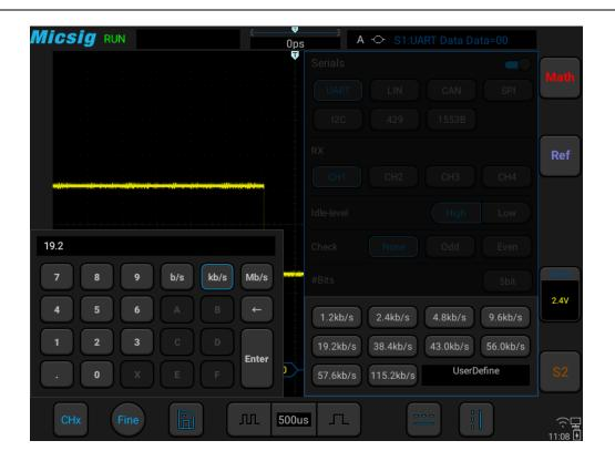
Figure 12-5 Baud Rate Default Setting
