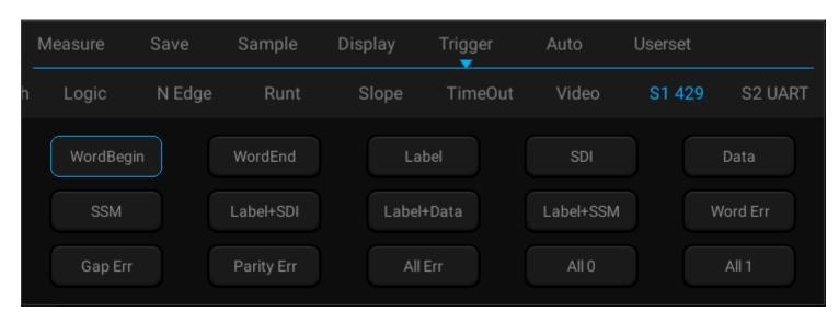
Figure 12-27 ARINC429 Trigger Mode Configuration Menu
