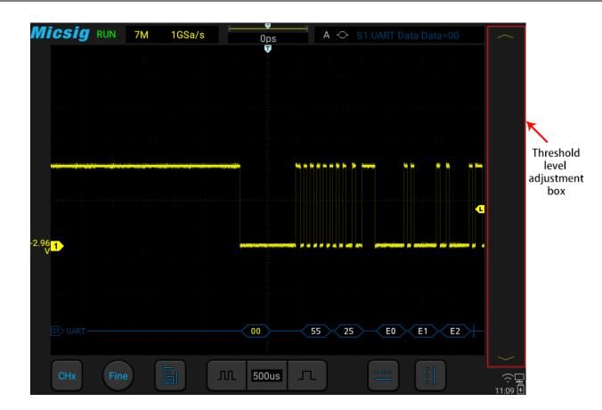
Figure 12-7 UART Decode Level Adjustment
