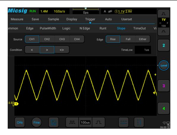
Figure 6-27 Slope Trigger Setting Menu
