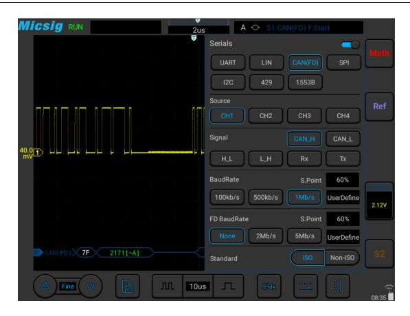
Figure 12-14 CAN / CAN FD Bus Configuration Menu
