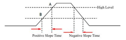
Figure 6-26 Positive/Negative Slope Time
