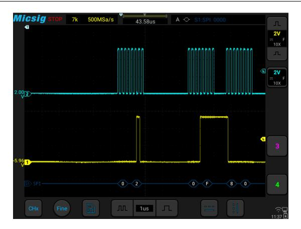
Figure 12-20 SPI Graphic Interface
