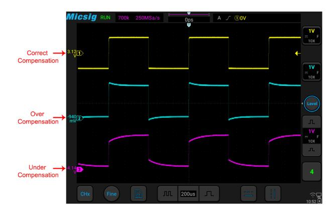
Figure 2-14 Probe Compensation
