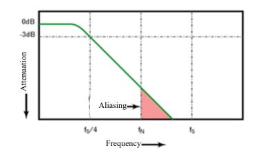
Figure 11-3 Sampling Rate and Oscilloscope Bandwidth
