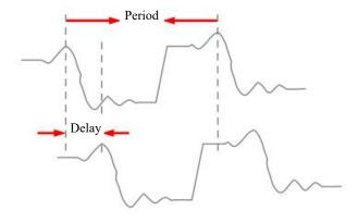
Figure 7-6 Phase Measurement Schematics
