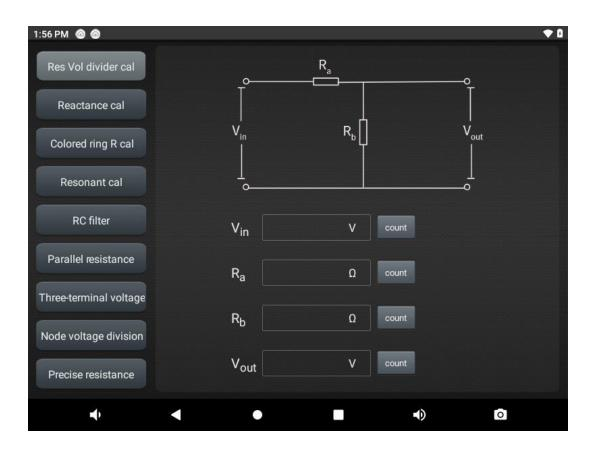
Figure 13-10 Electronic Calculation Tool Function
