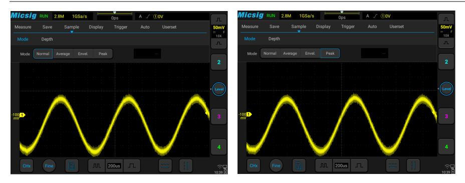
Figure 11-5 Sine Wave with Burr
