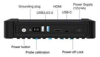
Power button, Grounding plug, Probe Calibration Output, USB3.0/2.0, HDMI, USB-C, Power Supply, Power-off Lock (Note: switch to ON for first-time use)
