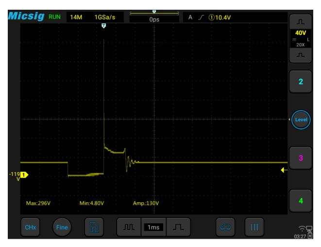
Figure 3-41 Primary ignition actual test
