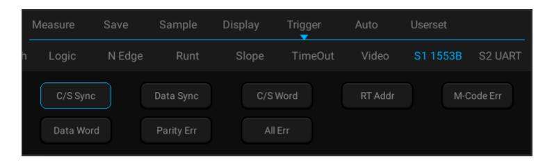
Figure 13-31 1553B Trigger Mode Configuration Menu
