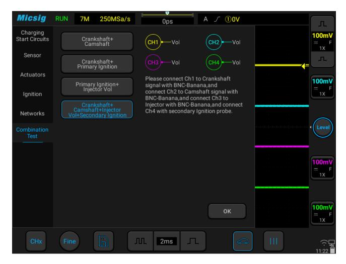
Figure 3-53 Combination test of Crankshaft + Camshaft + Injector + Secondary ignition
