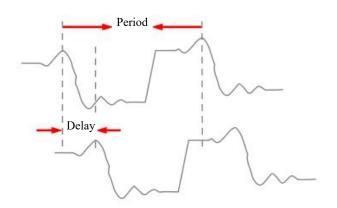
Figure 8-6 Phase Measurement Schematics
