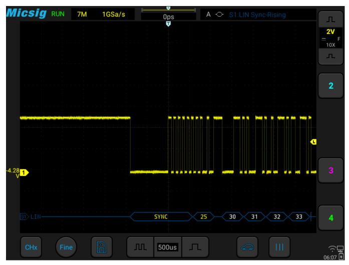
Figure 3-47 Audi A6 LIN bus measurement
