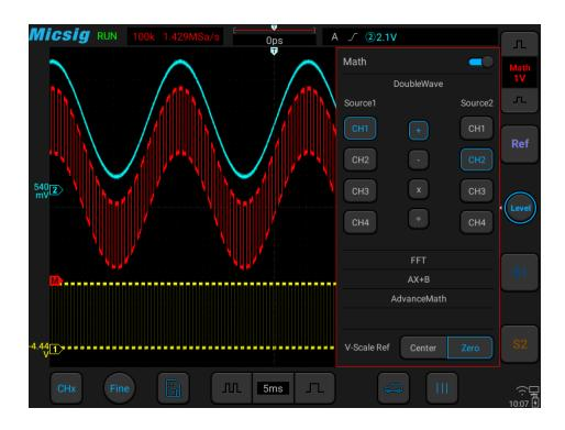
Figure 10-2 Mathematical Operation of CH1 adding CH2
