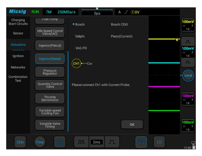
Figure 3-33 injector (diesel engine) test
