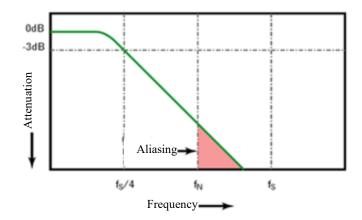
Figure 12-3 Sampling Rate and Oscilloscope Bandwidth
