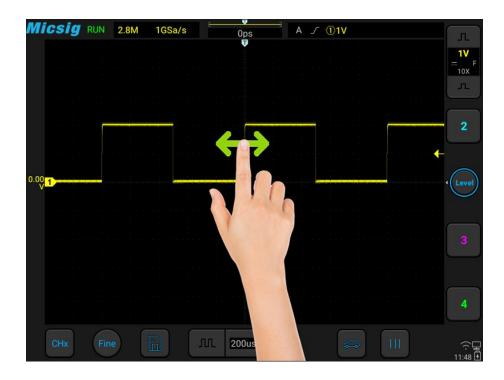
Figure 5-2 Move the Waveform Horizontally on the Screen
