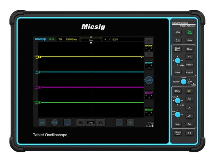
Figure 2-5 Front Panel of Tablet Oscilloscope
