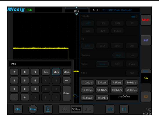
Figure 13-5 Baud Rate Default Setting
