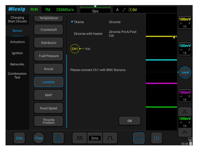
Figure 3-20 Lambda (oxygen sensor) test
