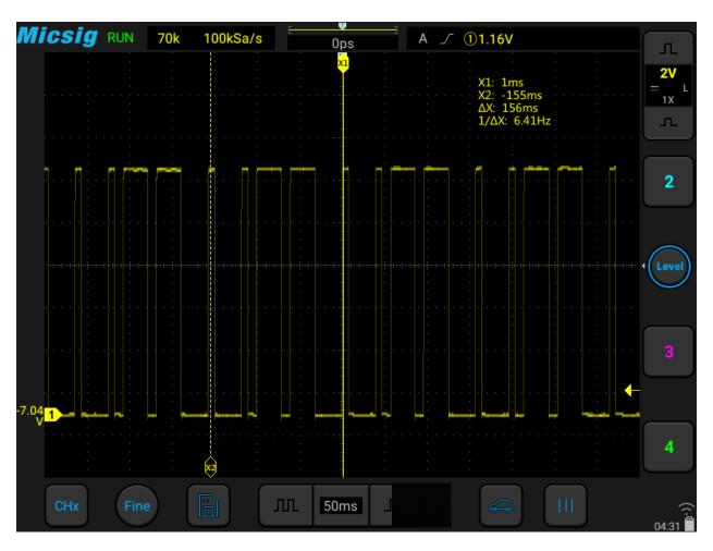
Figure 3-14 Camshaft position sensor (Hall type)
