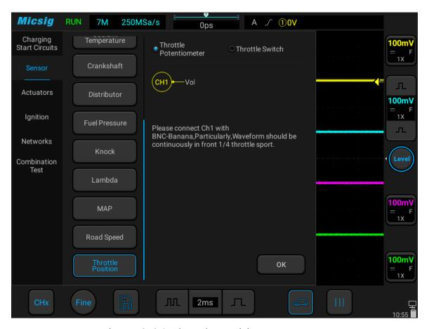
Figure 3-24 Throttle Position Sensor test
