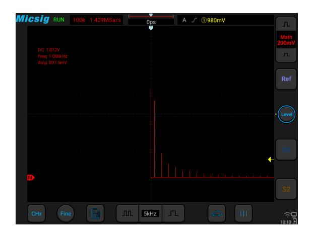
Figure 10-4 Spectrum Amplitude as V-Hz
