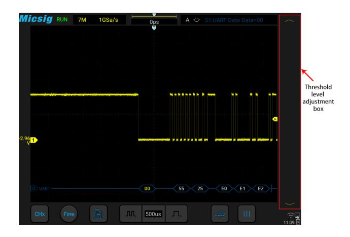
Figure 13-7 UART Decode Level Adjustment
