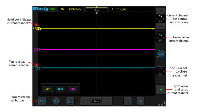
Figure 6-4 Channel Open, Close and Switching
