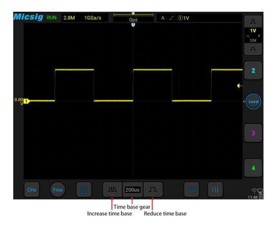
Figure 5-3 Adjust the Horizontal Time Base
