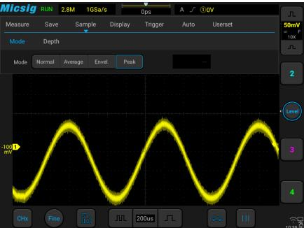
Figure 12-5 Sine Wave with Burr
