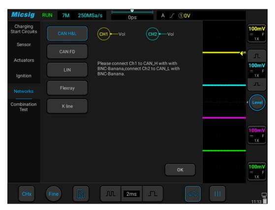
Figure 3-45 CAN BUS Test
