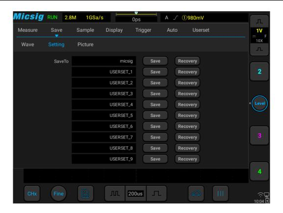
Figure 9-7 oscilloscope setting save
