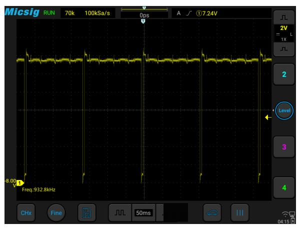
Figure 3-27 Audi A6 Carbon canister solenoid valve signal
