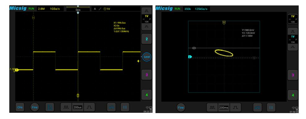
Figure 8-12 Cursor Measurement Pulse Width
