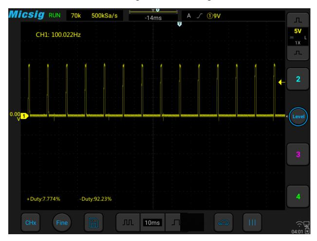
Figure 3-38 Cooling fan measurement diagram
