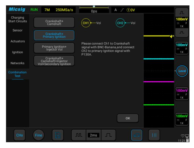
Figure 3-51 Crankshaft + Primary ignition test
