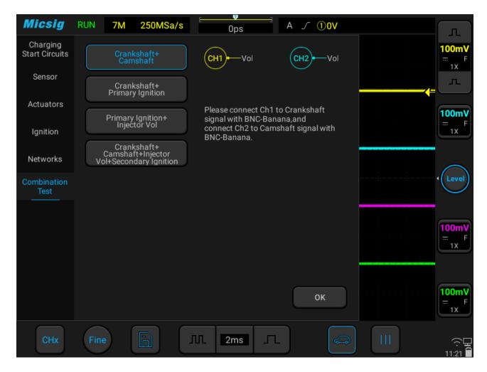
Figure 3-50 Crankshaft + Camshaft Combination Test
