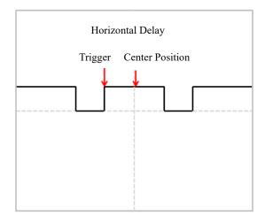
Figure 7-7 Horizontal Delay
