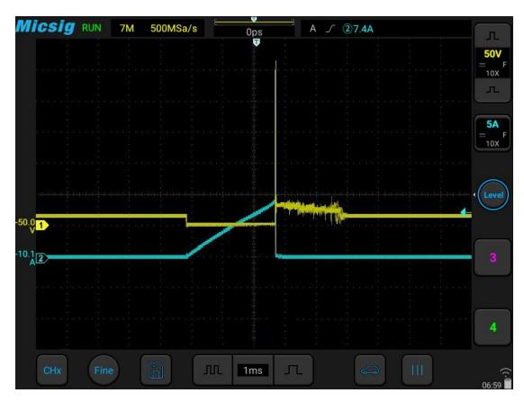
Figure 3-44 BMW 5 Series N20 Primary + Secondary ignition signal
