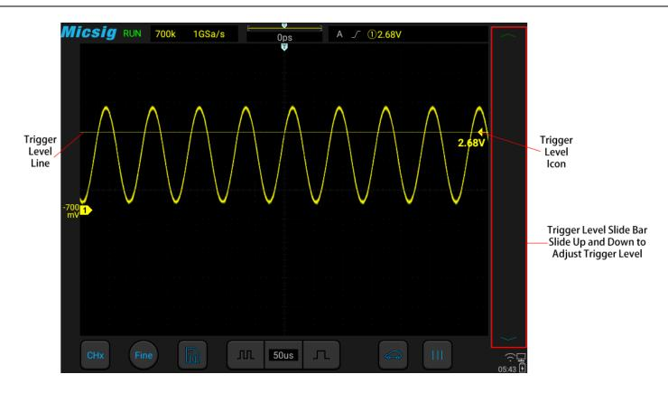
Figure 7-8 Trigger Level
