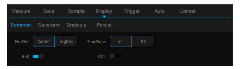
Figure 5-7 Roll Mode On/Off
