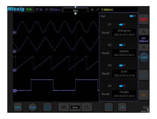
Figure 10-7 Restore Reference Waveform
