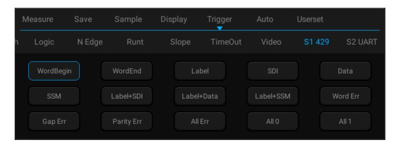
Figure 13-27 ARINC429 Trigger Mode Configuration Menu
