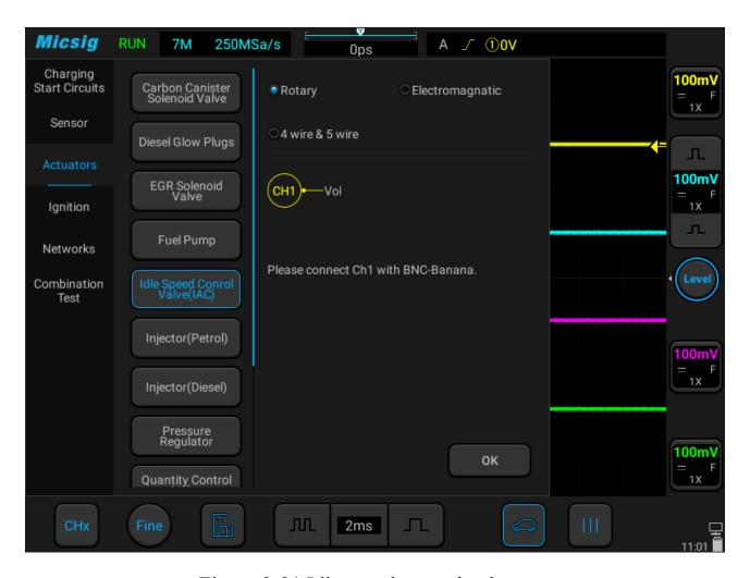
Figure 3-31 Idle speed control valve test
