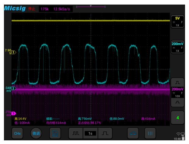
Figure 3-21 Lambda (Oxygen Sensor) diagram
