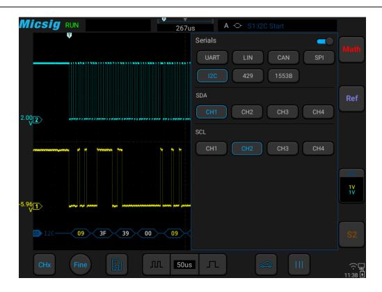
Figure 13-22 I2C Bus Configuration Menu
