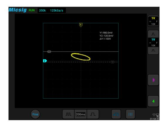
Figure 5-10 Phase Difference Measurement and Using the Cursor
