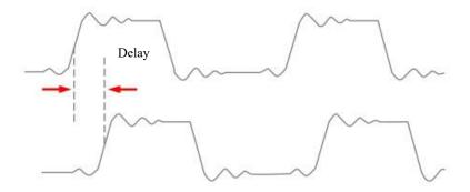
Figure 8-5 Delay Measurement Schematics
