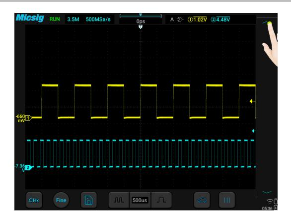
Figure 7-22 Trigger Level Adjustment
