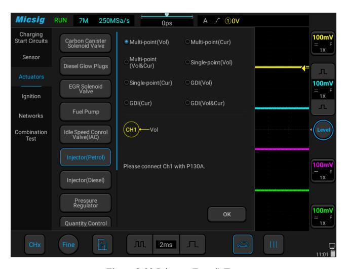
Figure 3-32 Injector (Petrol) Test
