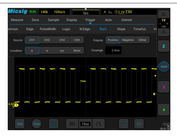
Figure 7-25 Runt Trigger Setting Menu
