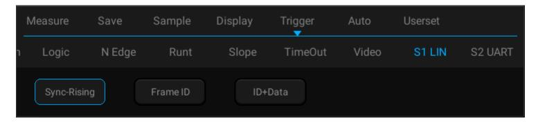
Figure 13-11 LIN Trigger Mode Configuration Menu
