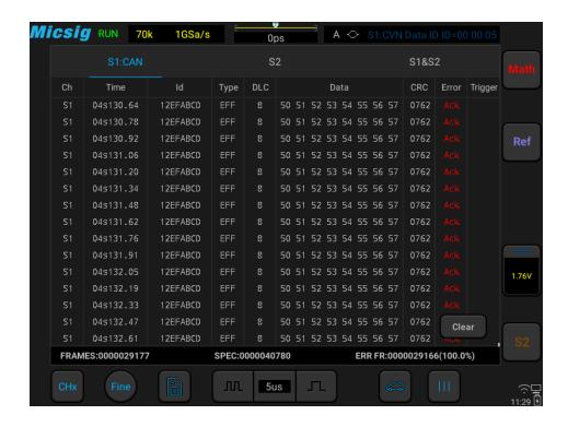
Figure 13-17 CAN Text Interface
