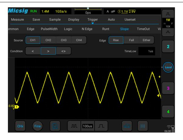
Figure 7-27 Slope Trigger Setting Menu
