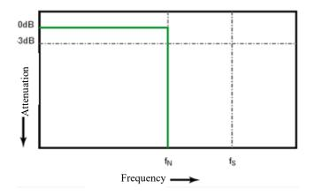
Figure 12-2 Theoretical Brick-Wall Frequency Response
