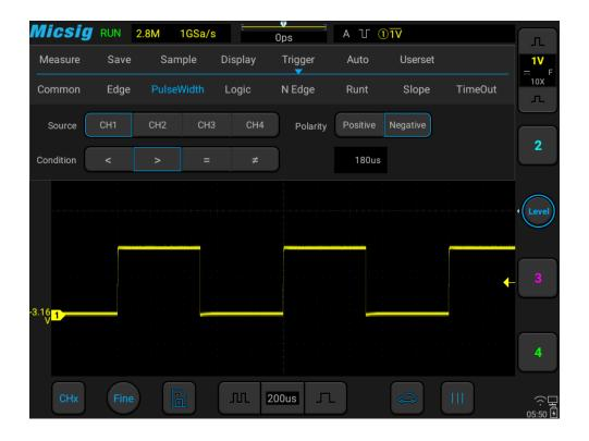
Figure 7-15 Negative Polarity Pulse Level Flip
