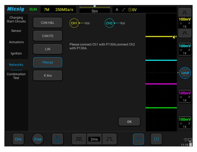
Figure 3-48: FlexRay bus test
