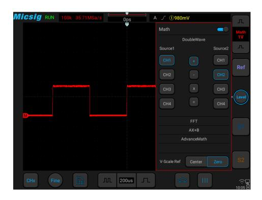
Figure 10-1 MATH Channel Waveform
