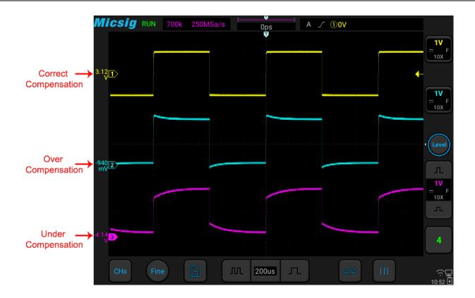
Figure 2-14 Probe Compensation
