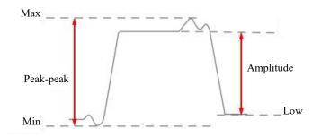
Figure 8-7 Voltage Measurement
