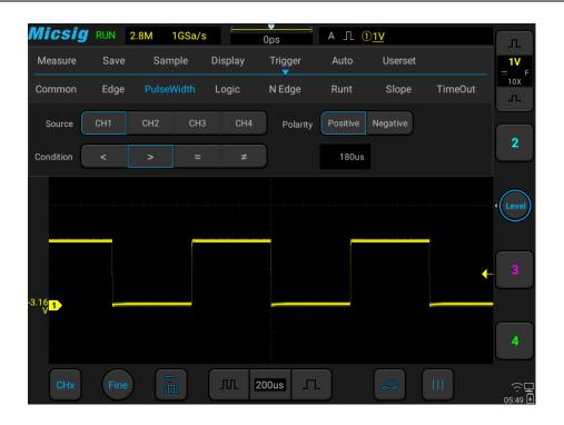
Figure 7-14 Pulse Width Trigger Setting Menu
