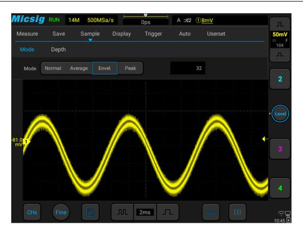
Figure 12-8 AM Signal in Envelope Sampling Mode (32)
