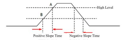
Figure 7-26 Positive/Negative Slope Time
