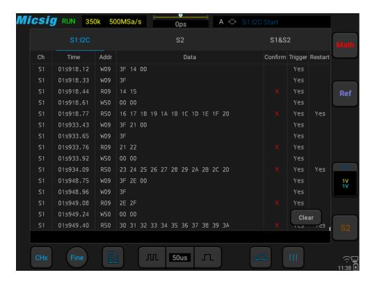
Figure 13-25 I2C Text Interface
