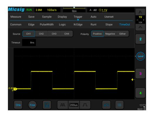
Figure 7-29 Time-out Trigger
