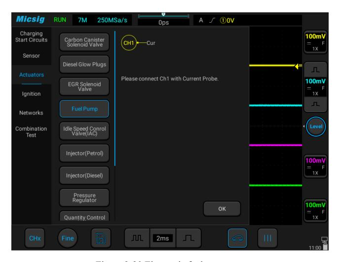
Figure 3-30 Electronic fuel pump test
