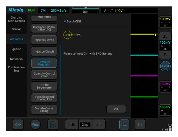
Figure 3-34 Pressure Regulator test
