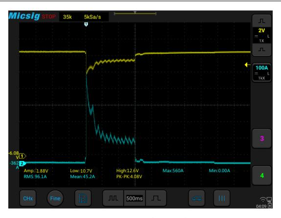
Figure 3-7 Starting voltage and current
