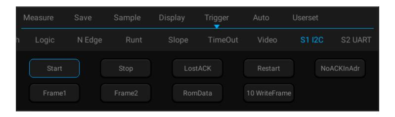
Figure 13-23 I2C Trigger Mode Configuration Menu
