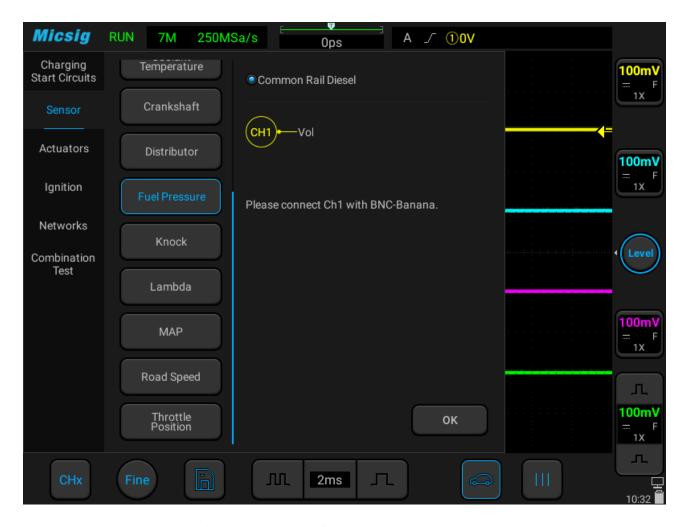
Figure 3-18 Fuel Pressure Sensor Test
