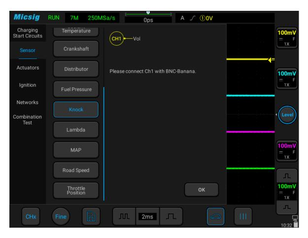
Figure 3-19 Knock Sensor test
