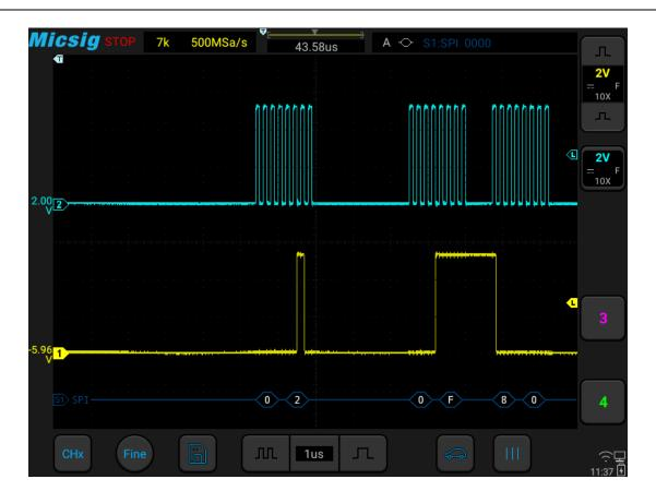
Figure 13-20 SPI Graphic Interface
