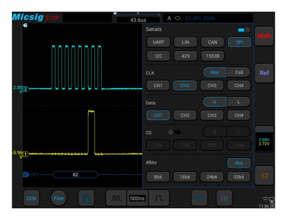
Figure 13-18 SPI Bus Configuration Menu
