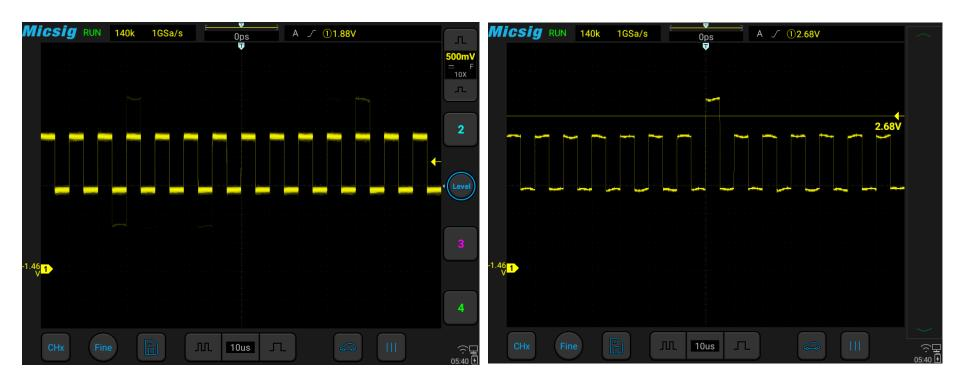
Figure 7-3 Abnormal Signal in Periodic Signals
