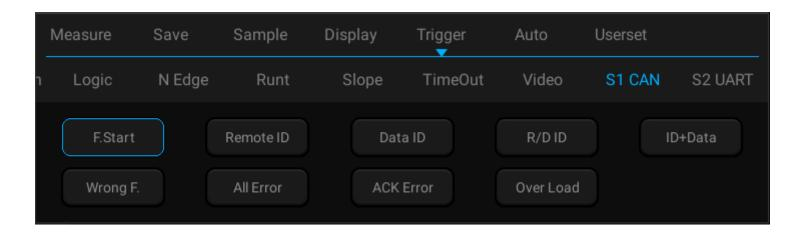
Figure 13-15 CAN Trigger Mode Configuration Menu
