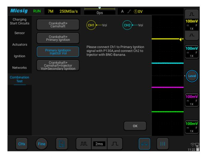
Figure 3-52 Primary ignition + Injector voltage
