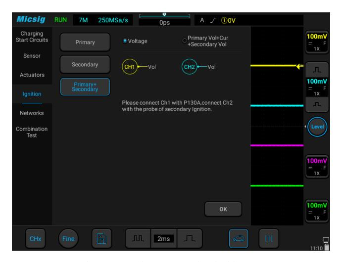
Figure 3-43: Primary + Scondary ignition test
