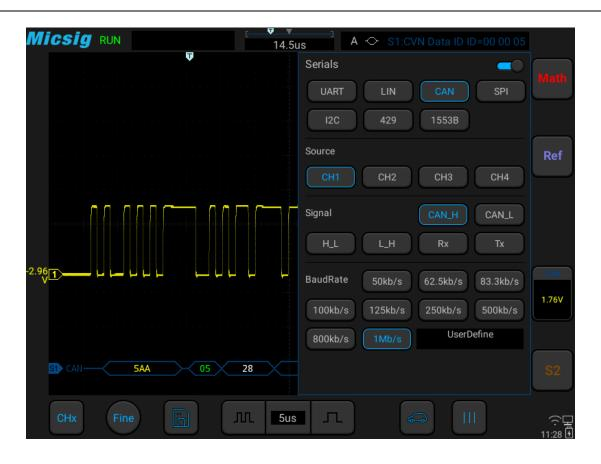
Figure 13-14 CAN Bus Configuration Menu
