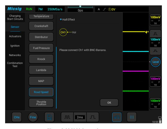
Figure 3-23 Vehicle speed sensor test
