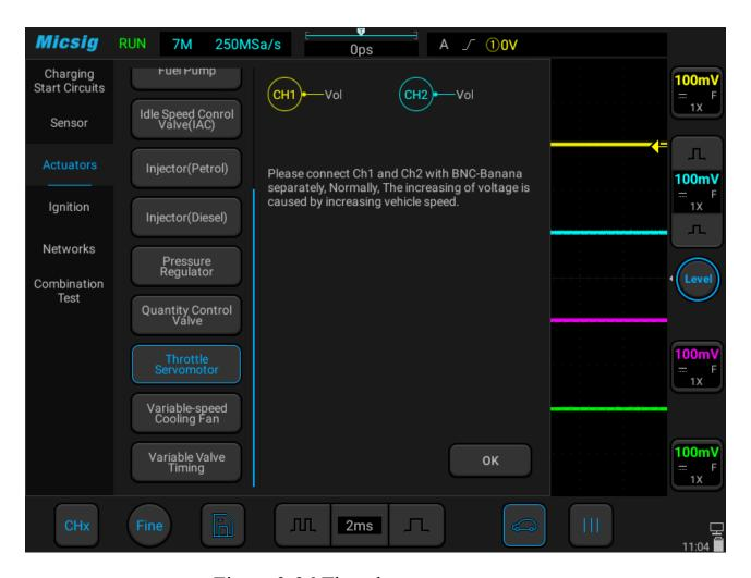
Figure 3-36 Throttle servo motor test
