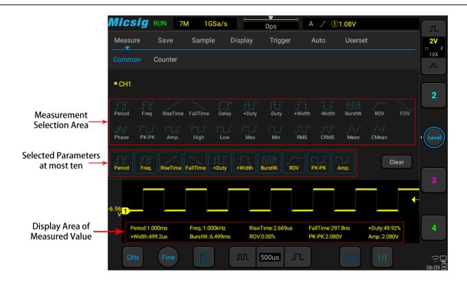
Figure 8-1 Automatic Measurement Menu
