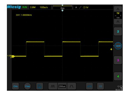
Figure 8-9 Frequency Meter Measurement
