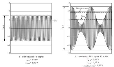
Because the RMS level of the modulated signal must match the test level, the peak amplitude of the modulated signal must be 5.1 dB greater than the RMS amplitude of the test level specified by the standard.
