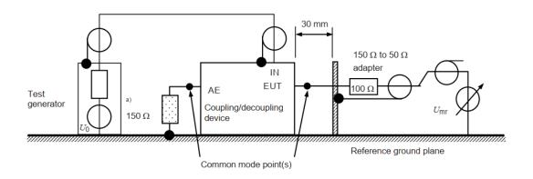
Voltage division factor RF-port to EUT-port: 150 kHz - 80 MHz: 9.5 dB  $\pm$  1dB 80 MHz - 230 MHz: 9.5 dB +3 dB / - 2 dB
