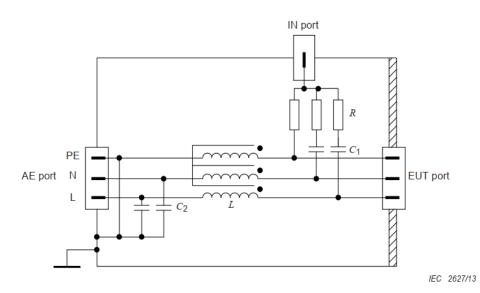
CDN-M3,  $C_1$  (typical) = 10 nF,  $C_2$  (typical) = 47 nF,  $R = 300 \Omega$ ,  $L \ge 280 \mu$ H at 150 kHz CDN-M2,  $C_1$  (typical) = 10 nF,  $C_2$  (typical) = 47 nF,  $R = 200 \Omega$ ,  $L \ge 280 \mu$ H at 150 kHz CDN-M1,  $C_1$  (typical) = 22 nF,  $C_2$  (typical) = 47 nF,  $R = 100 \Omega$ ,  $L \ge 280 \mu$ H at 150 kHz
