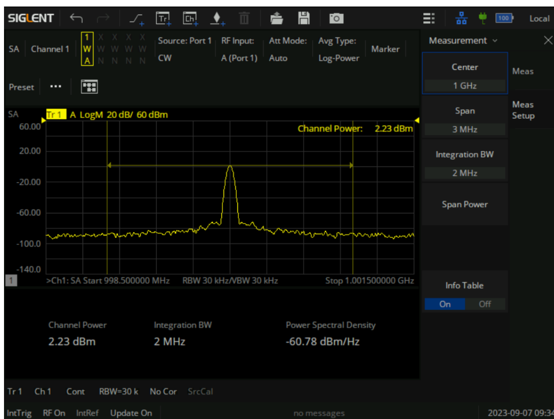
Figure 9-12 Channel Power measure
