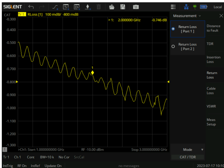
Figure 11-7 Return loss measurement interface
