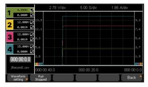
The SPD4000X series programmable linear DC power supply is equipped with a 4.3-inch, true color TFT-LCD display screen with a resolution of 480×272. 4 channels of voltage and current waveform run chart can be set, allowing users to dynamically observe changes in the output state more intuitively.
