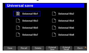
The power supply allows users to save multiple types of files to memory for later recall. The power supply provides a non-volatile internal memory and access to external memory via the USB Host interface on the rear panel. Save setups, settings, and more directly to the supply or to a USB memory stick for transport.
