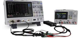
The SDS5000X can control the USB AWG module or a standalone SIGLENT SDG generator, to scan the amplitude and phase frequency response of the DUT, and display the data as a Bode Plot. This makes it possible to replace expensive network analyzer in some applications
