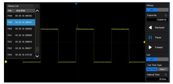
History function can record up to 100,000 frames of waveforms. The recording is executed automatically, so that the customer can play back the history waveforms at any time in order to observe unusual events and quickly locate the area of interest using the cursors or measurements. The failed frames of Mask Test can be stored as history
