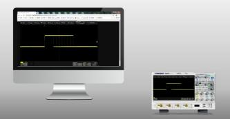
With the embedded web server, users can control the oscilloscope from a simple web page. This provides wonderful remote troubleshooting and monitoring capabilities
