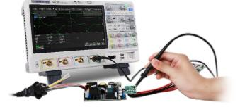
The Power Analysis option provides a full suite of power measurements and analysis, which greatly improve the measurement efficiency in switching power supplies and power devices design
