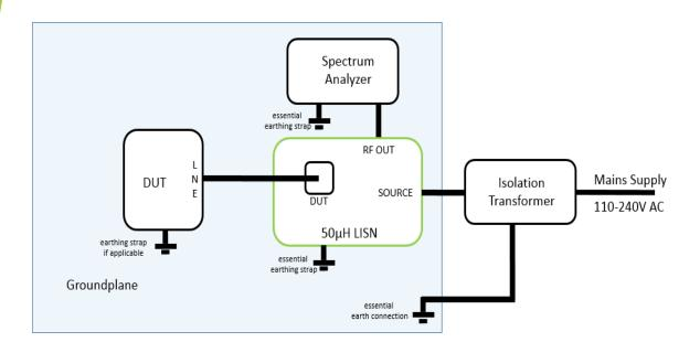
The DUT shall be isolated and elevated from the groundplane. The spectrum analyzer shall measure conducted emissions on both line and neutral.
