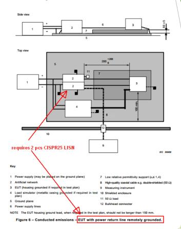
Applicable Tekbox 5µH LISN for conducted measurements at supply terminals: TBOH01 or TBL0550-1
