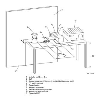
Measurement set up example taken from CISPR 16:
