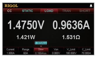
Current rising speed is defined as the speed of transition from one setting to another. You can set the actual transition time from one setting to another by changing the current rising speed. Adjustable current rising speed: 0.001 A/ $\mu$ s to 5 A/ $\mu$ s.
