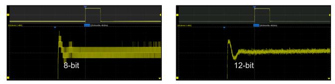
Vertical & Horizontal Zoom along with a large memory depth make the most out of 12-bit ADC resolution. Engineers can observe waveform overall and details simultaneously.
