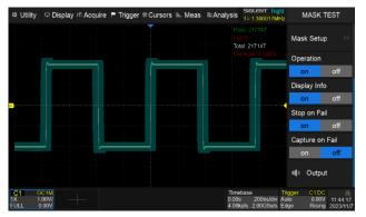
The oscilloscope utilizes a hardware-based Mask Test function, performing up to 80,000 Pass / Fail decisions each second. It is easy to generate user-defined test templates to provide trace mask comparisons, making it suitable for long-term signal monitoring or automated production line testing.
