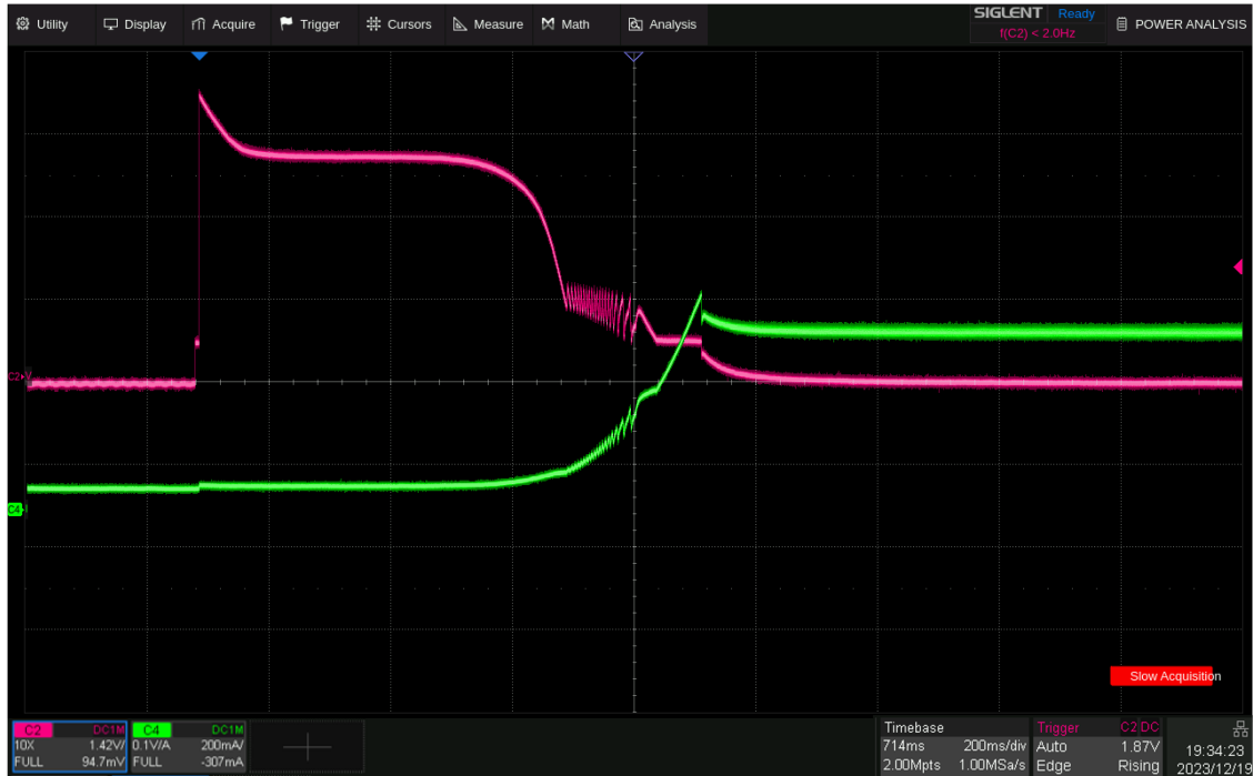
Voltage and current waveforms on the MOSFET at power-up
