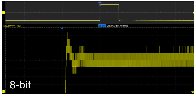
12-bit resolution shows you more details and less noise on the waveform.
