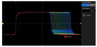
Segmented memory collection will store the waveform into multiple memory segments (up to 80,000) and each segment will store a triggered waveform as well the dead time information. The interval between segments can be as small as 2 µs. All of the segments can be played back using the History function.
