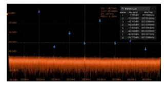
Hardware-accelerated FFT supports up to 2 Mpts operation. This provides high-frequency resolution with a fast refresh rate. The FFT function also supports a variety of window functions so that it can adapt to different spectrum measurement needs. Three modes (Normal, Average, and Max hold) can satisfy different requirements for observing the power spectrum. Auto peak detection and markers are supported.
