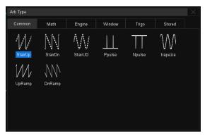
The USB waveform generator can output waveforms with up to 25 MHz frequency and  $\pm 3$  V amplitude. Six basic waveforms together with multiple types of predefined waveforms and as user-defined arbitrary waveforms are supported.
