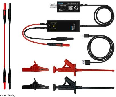
\* Extension leads, twist together can lower noise
