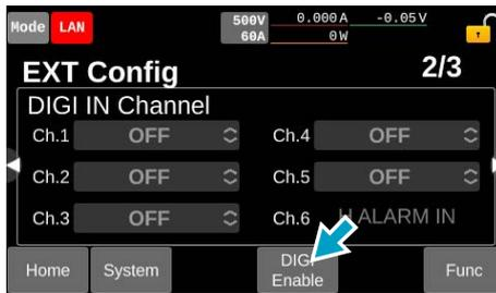
Enable the digital input/output.
