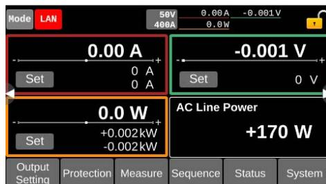
By factory default, the panel settings immediately before the POWER switch is turned off are saved. When you turn the power on, the product starts in the same state as it was in the last time it was turned off.
