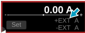
Due to Setting the Output Mode (p.49), the values cannot be changed from the display during external control (EXT), pulse function operation (PULSE), sine function operation (SINE), or I-V characteristic function operation (I-V).
