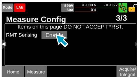
When remote sensing is enabled, the sensing icon (
