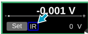
CV is set to IR in "Setting the Output Mode" (p.49).
