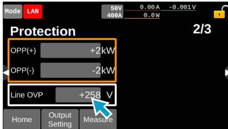
Input voltage rating 200 Vac model: 200 V to 258 V
