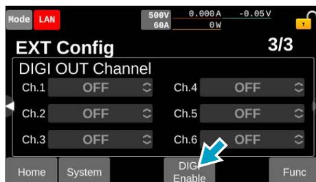
Enable the digital input/output.
