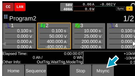
Trigger wait is released for all PXB series to be synchronized, and sequence resumes simultaneously.
