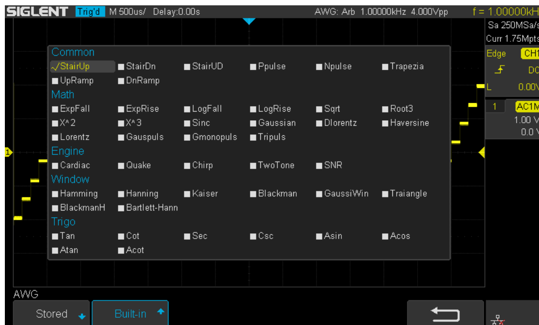
Figure 117 Built-in Arb Interface
