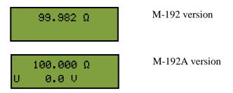
In the upper row generated resistance in  $[\Omega]$  is displayed. In the lower row mesaured voltage connected to the output terminals (M-192A only) is displayed.
