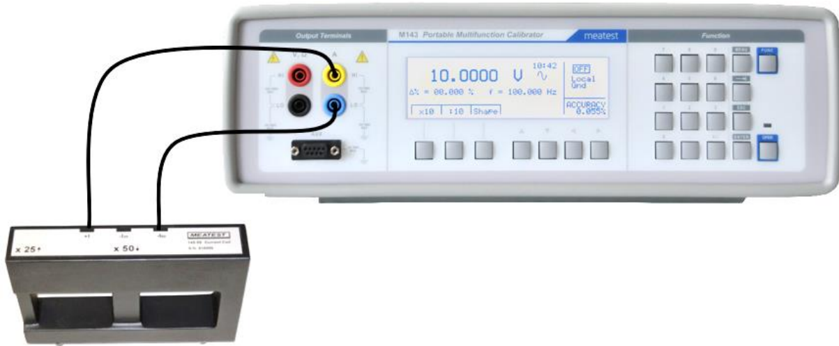
Figure 7 Current coil connection
