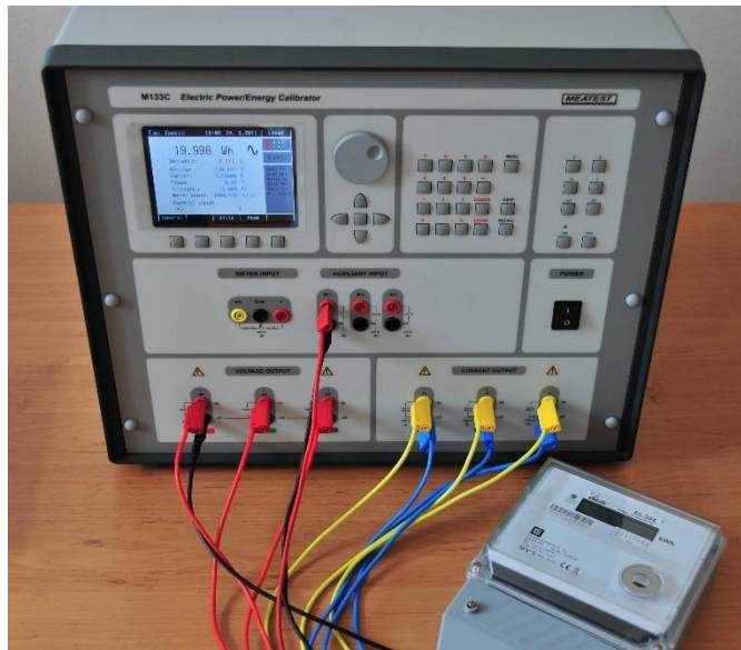
Figure 23 Energy meter calibration example
