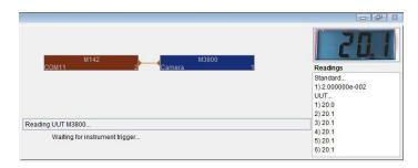
The program is suitable for the checking of measuring instruments because it enables an elaboration of multiple measurements, calculation of the value dispersion as well as measurement uncertainty.
