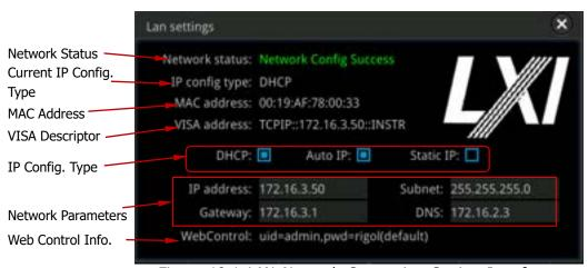
Figure 19-1 LAN Network Connection Setting Interface
