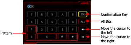
Figure 5-6 Virtual Keypad for Pattern Setting
