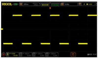
Figure 4-2 Waveforms before Averaging
