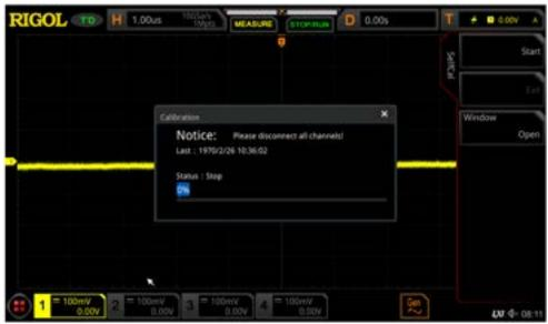
Figure 19-2 Self-calibration Interface
