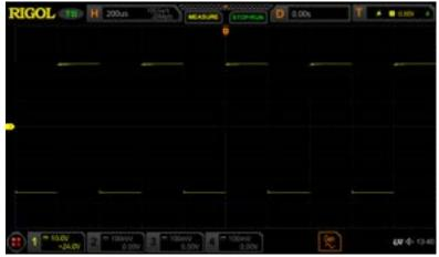
Figure 4-3 Waveforms after 128 Times of Averaging
