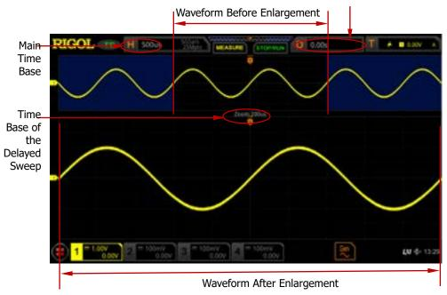
Figure 3-1 Delayed Sweep Mode
