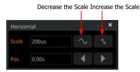
You can click on the function navigation icon to open the function navigation. Then click **Acquisition** → **Fine** to enable or disable the fine adjustment of the horizontal time base.
