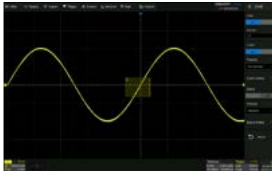
Select C1 as the source, turn on zone1, and set the property as "Not Intersect"
