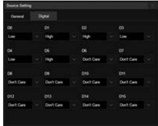
The logical setting of digital channels
