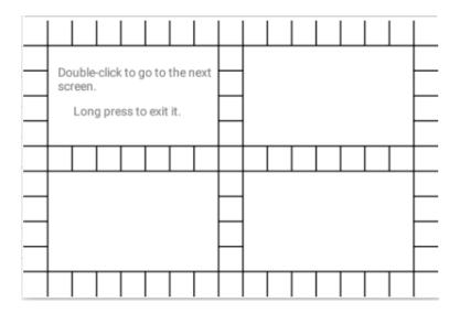
Double-click the current test screen or tap the screen twice to go to the next test screen. Also when all the boxes have turned green, it will go to the next test screen automatically, as shown in the figure below. At this time, you can pinch or stretch the RIGOL icon to zoom it out or in to check whether the touch-enabled gestures work normally. Long press the screen to exit the test interface.
