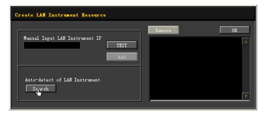
Besides, you can input the IP address of the instrument manually into the text field under "Manual Input LAN Instrument IP", then click **TEST**. If the instrument passes the test, click **ADD** to add the instrument to the LAN instrument resource list in the right section; if the instrument fails the test, please check whether the IP address that you input is correct, or auto search the IP address of the instrument and add it to the instrument resource.
