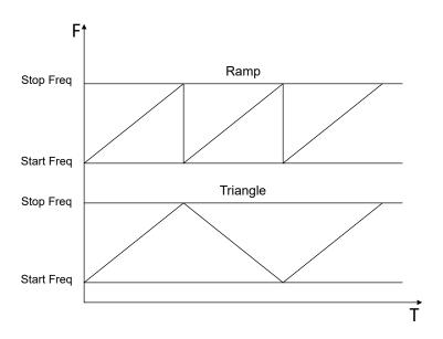
Figure 8.1 Diagram of the Sweep Shape in "Fwd" Sweep Direction
