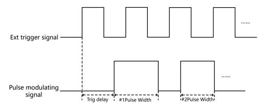
Figure 9.2 Trigger Delay
