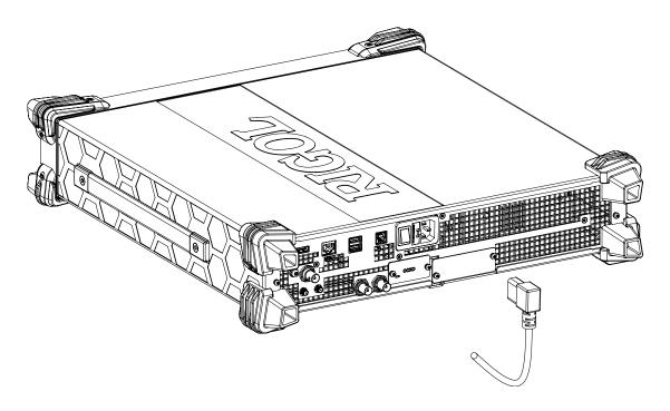
**Figure 4.5 To Connect to AC Power**
