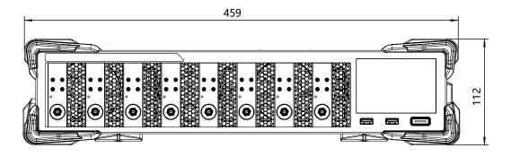
Figure 4.1 Front View (Unit: mm)
