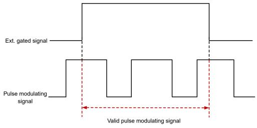
To specify the polarity of the external gated signal, click or tap **Gate Polar** to select "Normal" or "Inverted". By default, it is "Inverted".
