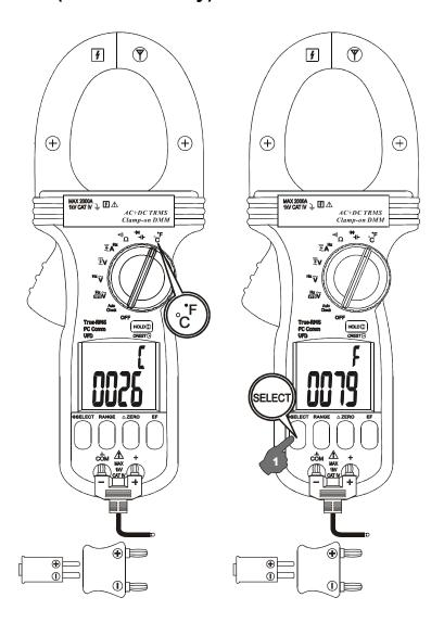
Defaults at °C (Celsius) readings. Press SELECT button momentarily and release to select °F (Fahrenheit) readings. Inputs are made through the test leads terminals. Be sure to insert the banana plug type-K temperature bead probe Bkp60 with correct + — polarities. You can also use a plug adapter Bkb32 (Optional purchase) with banana pins to type-K socket to adapt other type-K standard mini plug temperature probes.
