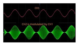
**Channel Modulation** One channel can modulate the other without external connections. This feature provides an easy method for complex modulation waveform creation. The modulating wave channel can be directly output and compared with the modulated signal.
