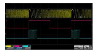
**Sweep and Burst** Sweep supports "Line" and "Log" modes, while Burst enables "NCycle" and "Gated" modes. Both Sweep and Burst support trigger sources: Internal, External, and Manual.
