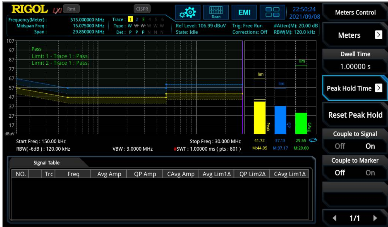
Figure 6: Adjustment of measurement meter with different detectors and coupled to signal
