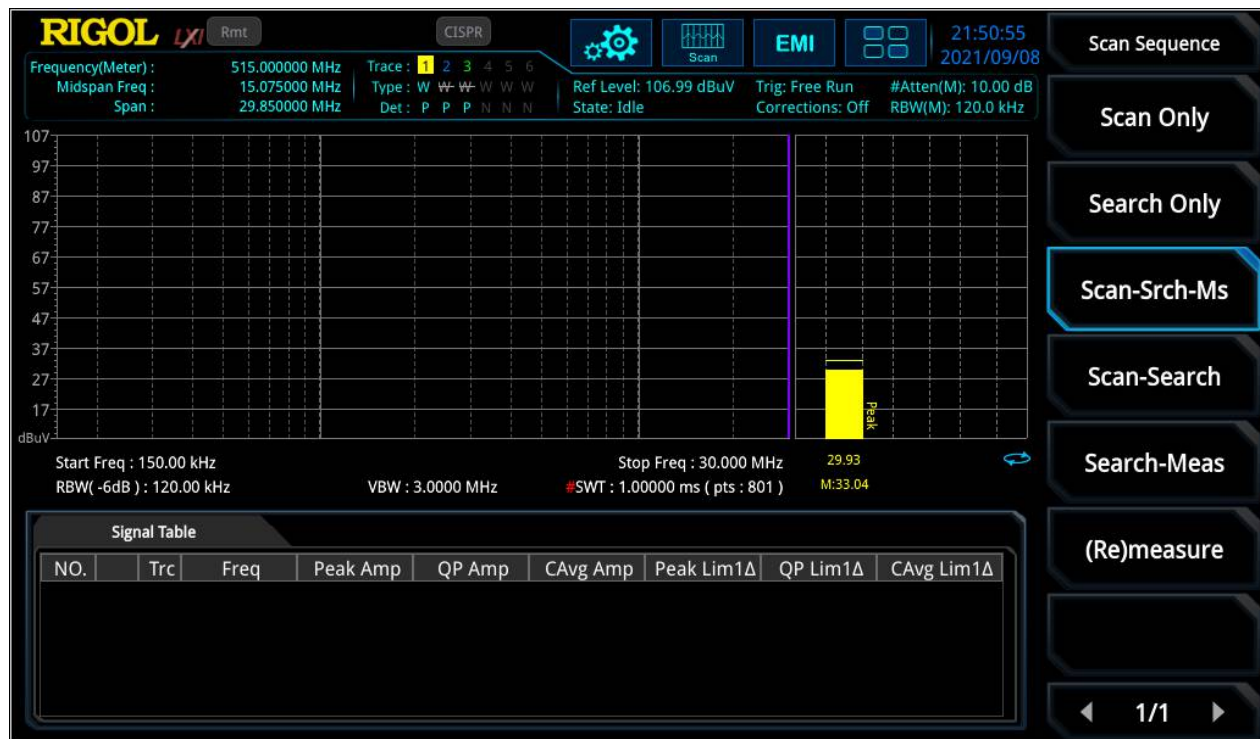
Figure 4: Scan Sequence adjustment with "Scan-Search-Measure"
