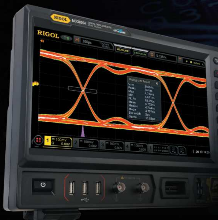
Perform eye measurement on the 622 Mb/s signal.
