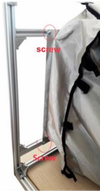
Picture 10: fabrics before attaching it to the frame
