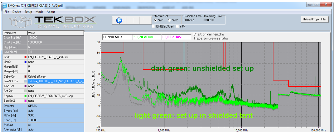
Picture 6: CISPR 25 conducted noise measurement; DUT powered
