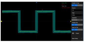
The SDS5000X utilizes a hardware-based Mask Test function, performing up to 18,000 Pass / Fail decisions each second. It is easy to generate user-defined test templates in order to provide trace mask comparisons, making it suitable for long-term signal monitoring or automated production line testing
