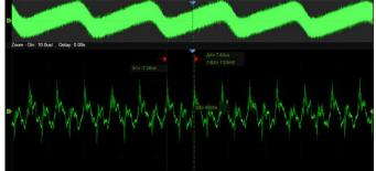
Using hardware-based Zoom technique and record length of up to 250 Mpts, users can select a slower timebase without compromising the sample rate, and then quickly zoom in to focus on the area of interest
