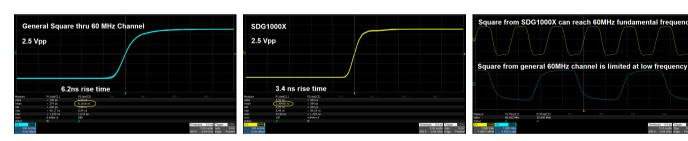
Benefitting from a special square-wave generating circuitry, the Square from the SDG1000X breaks the 60 MHz bandwidth barrier, reaching rise/fall times of less than 4.2 ns, and frequencies up to 60 MHz.
