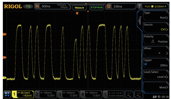
The Runt trigger helps you capture the runt pulse signal in the pulse train
