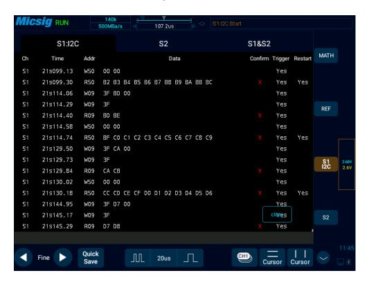
Figure 12-25 I2C Text Interface
