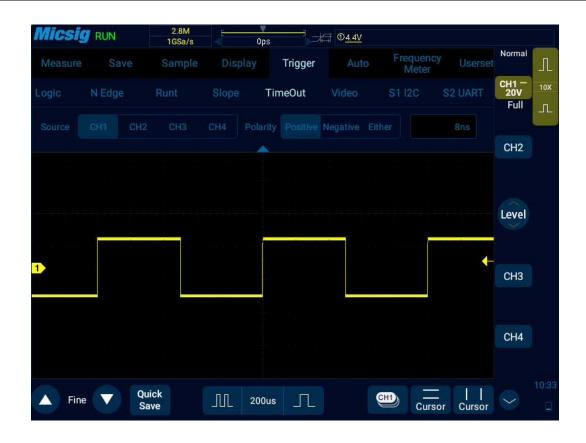
Figure 6-28 Time-out Trigger
