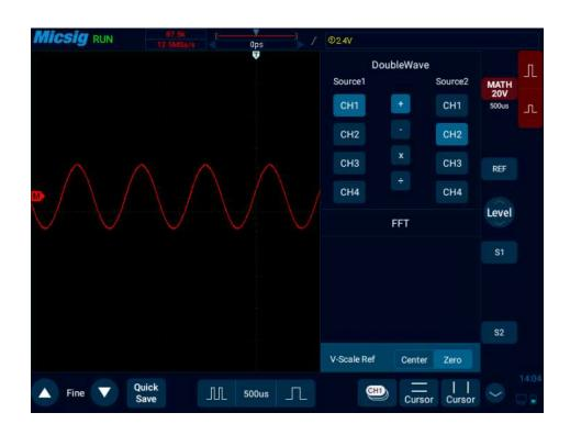
Figure 9-1 MATH Channel Waveform
