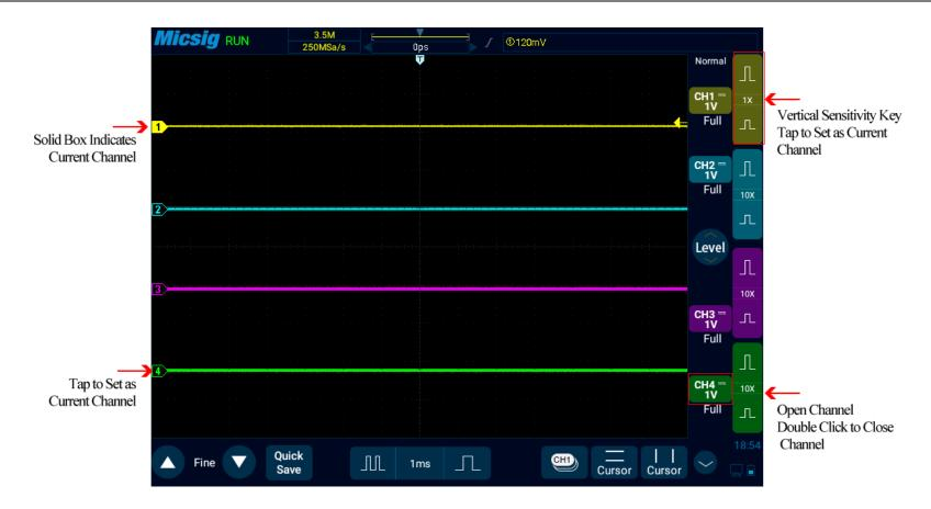
Figure 5-4 Channel Open, Close and Switching
