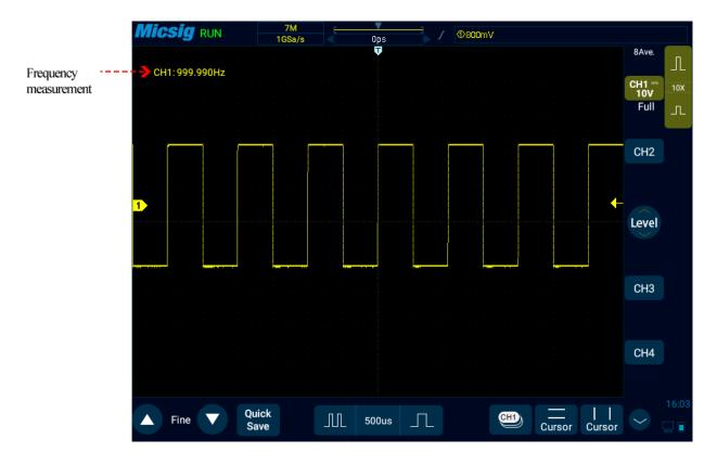
Figure 7-9 Frequency Meter Measurement
