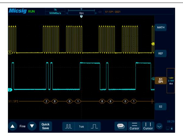
Figure 12-20 SPI Graphic Interface
