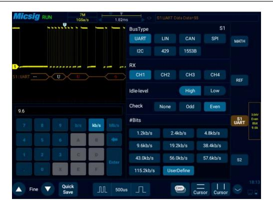
Figure 12-5 Baud Rate Default Setting
