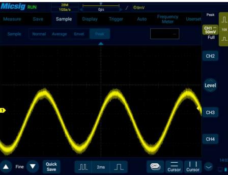
Figure 11-5 Sine Wave with Burr
