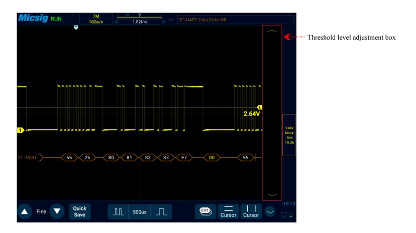
Figure 12-7 UART Decode Level Adjustment
