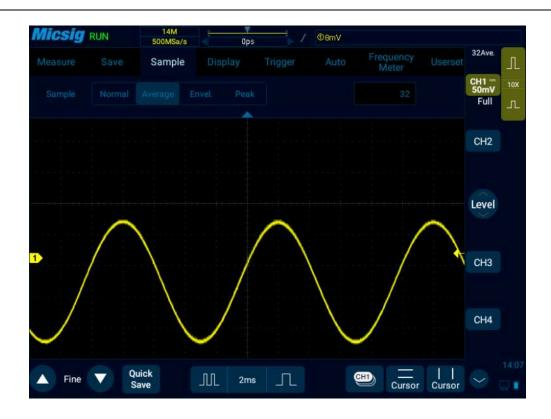
Figure 11-7 Waveform after choosing the average sampling mode, with average number 32
