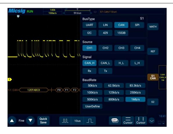
Figure 12-14 CAN Bus Configuration Menu
