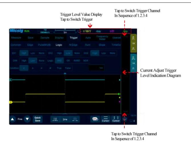
Figure 6-21 Trigger Level Adjustment
