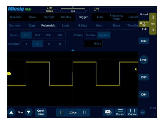
Figure 6-14 Negative Polarity Pulse Level Flip
