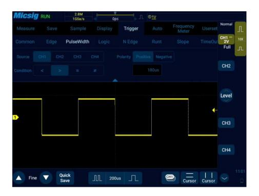
Figure 6-13 Pulse Width Trigger Setting Menu
