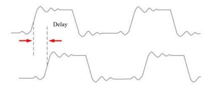
Figure 7-5 Delay Measurement Schematics
