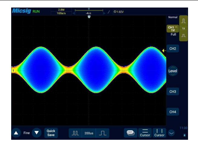
Figure 10-5 Color Temperature Open Mode
