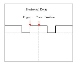
Figure 6-7 Horizontal Delay
