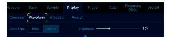
Figure 10-2 Waveform Display Menu
