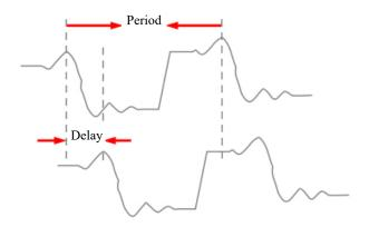
Figure 7-6 Phase Measurement Schematics
