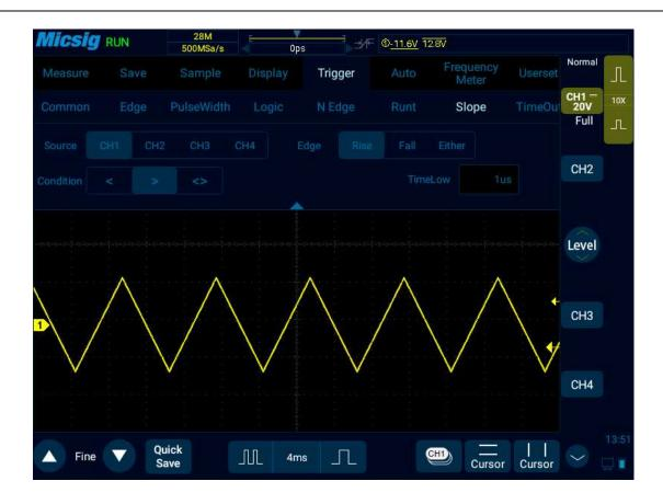
Figure 6-26 Slope Trigger Setting Menu
