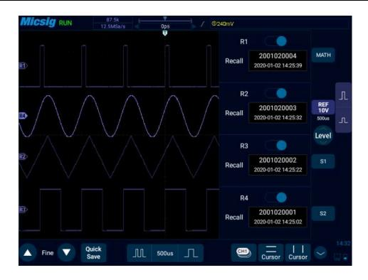
Figure 9-6 Restore Reference Waveform
