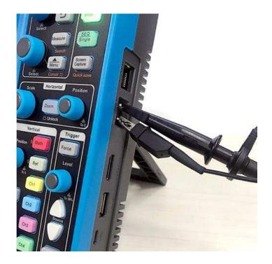
Figure 2-13 Probe Connection
