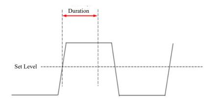
Figure 6-27 Timeout Trigger Schematics
