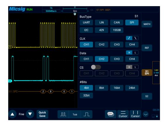
Figure 12-18 SPI Bus Configuration Menu
