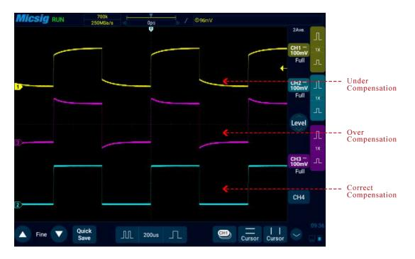
Figure 2-14 Probe Compensation
