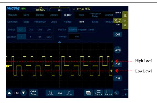
Figure 6-24 Runt Trigger Setting Menu
