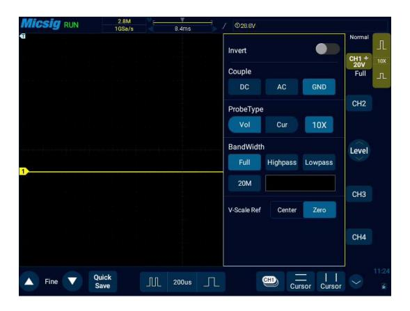
Figure 5-9 GND Coupling
