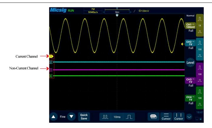
Figure 5-2 Current Channel and Non-Current Channel
