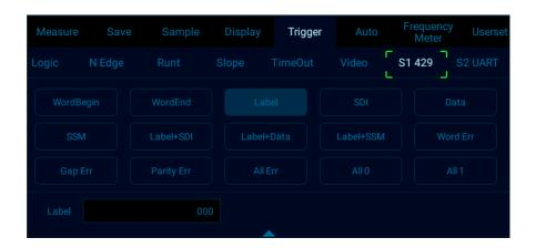
Figure 12-27 ARINC429 Trigger Mode Configuration Menu
