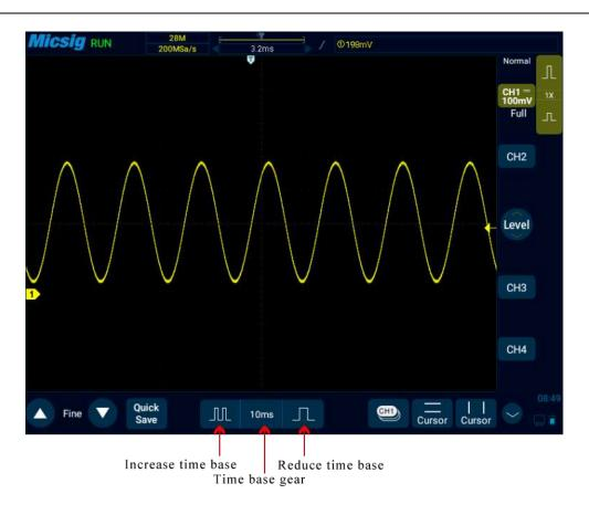
Figure 4-3 Adjust the Horizontal Time Base
