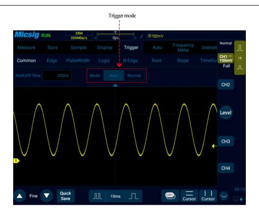
Figure 6-5 Oscilloscope Trigger Mode Setting
