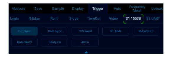
Figure 12-31 1553B Trigger Mode Configuration Menu
