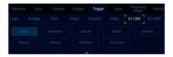
Figure 12-15 CAN Trigger Mode Configuration Menu
