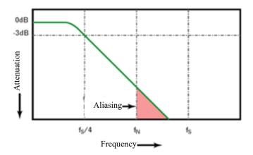
Figure 11-3 Sampling Rate and Oscilloscope Bandwidth
