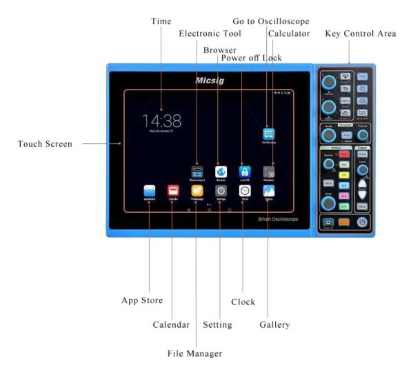
Figure 2-4 Front Panel of Tablet Oscilloscope
