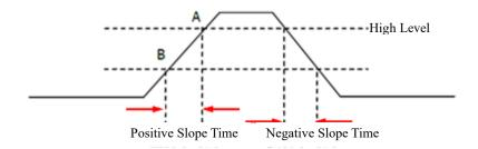
Figure 6-25 Positive/Negative Slope Time
