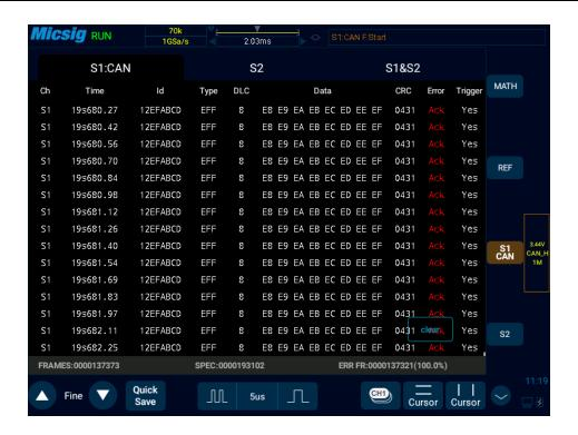
Figure 12-17 CAN Text Interface
