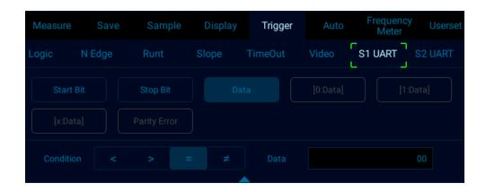
Figure 12-6 Trigger Setting Menu
