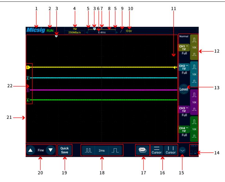
Figure 2-5 Oscilloscope Interface Display
