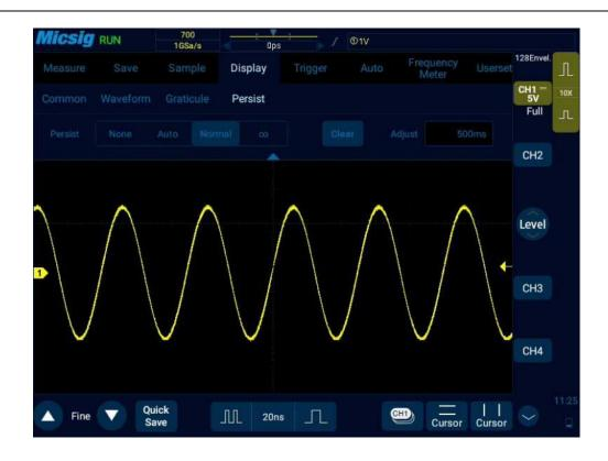
Figure 10-4 20MHz Sine Wave Variable Persist 500ms
