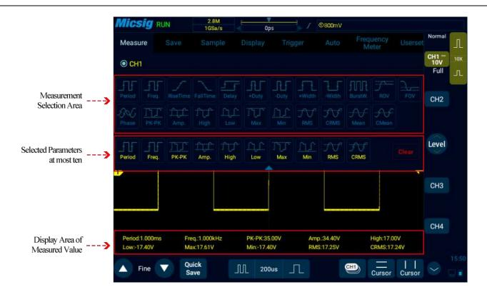
Figure 7-1 Automatic Measurement Menu
