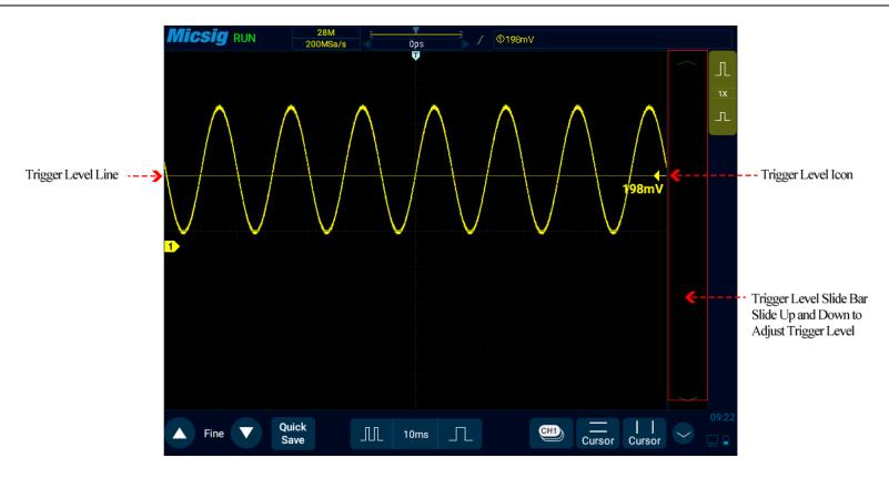
Figure 6-8 Trigger Level
