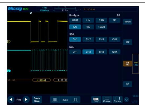
Figure 12-22 I2C Bus Configuration Menu
