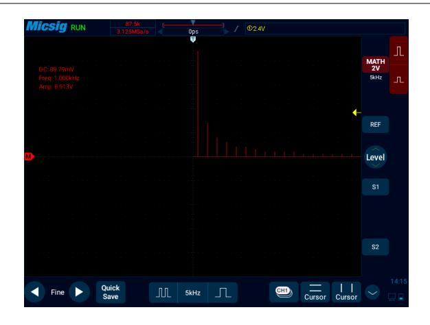
Figure 9-4 Spectrum Amplitude as V-Hz
