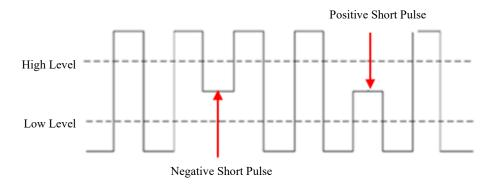
Figure 6-23 Runt Trigger
