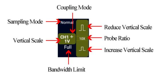
Figure 5-3 Channel Display Interface
