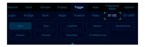
Figure 12-23 I2C Trigger Mode Configuration Menu
