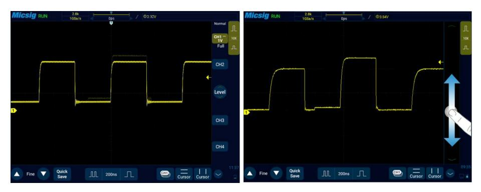
Figure 6-3 Abnormal Signal in Periodic Signals
