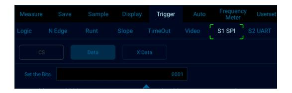
Figure 12-19 SPI Trigger Mode Configuration Menu
