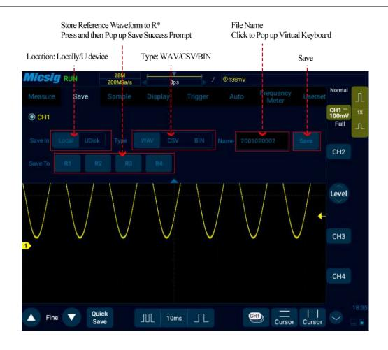
Figure 8-4 Save CH1 Reference Waveform Interface
