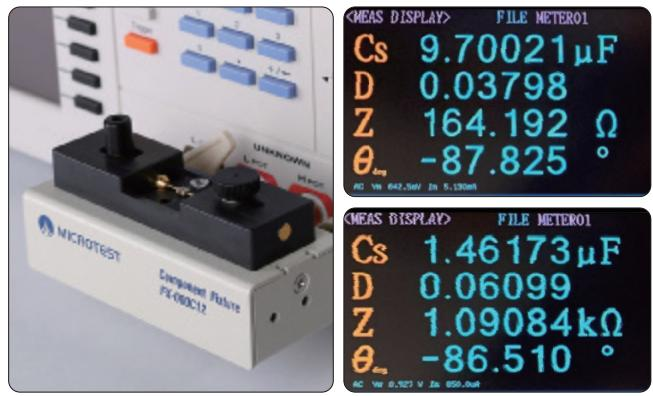
Evaluation of DC bias voltage characteristics with semiconductor wafer or ceramic multilayer capacitors
