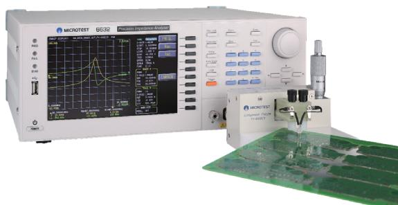
Testing PC board inductance coil
